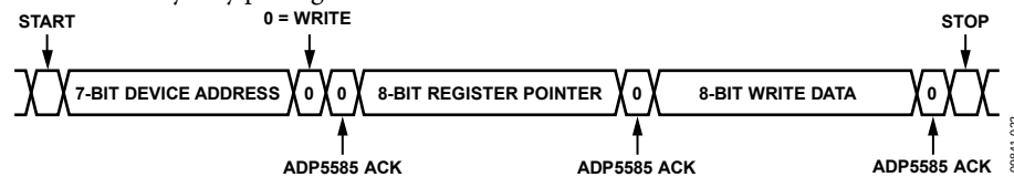
Figure 23. I 2 C Single Byte Write Sequence
