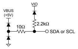
VIO is the programmed Target I/O voltage of the Adapter. The GP3/VDD pin has the following equivalent input circuit, assuming the pin is operating as GP3:
