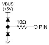
The SDA and SCL pins have the following equivalent input circuit (assuming the built-in  $2.2k\Omega$  pull-up resistors are disabled):
