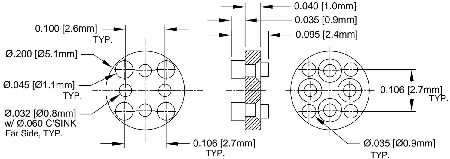
2. MATERIAL: NYLON 6/6, 94V-2, WHITE. BIVAR MATERIAL CODE 04-WE. BASF ULTRAMID NYLON 6/6 A3K WHITE.
