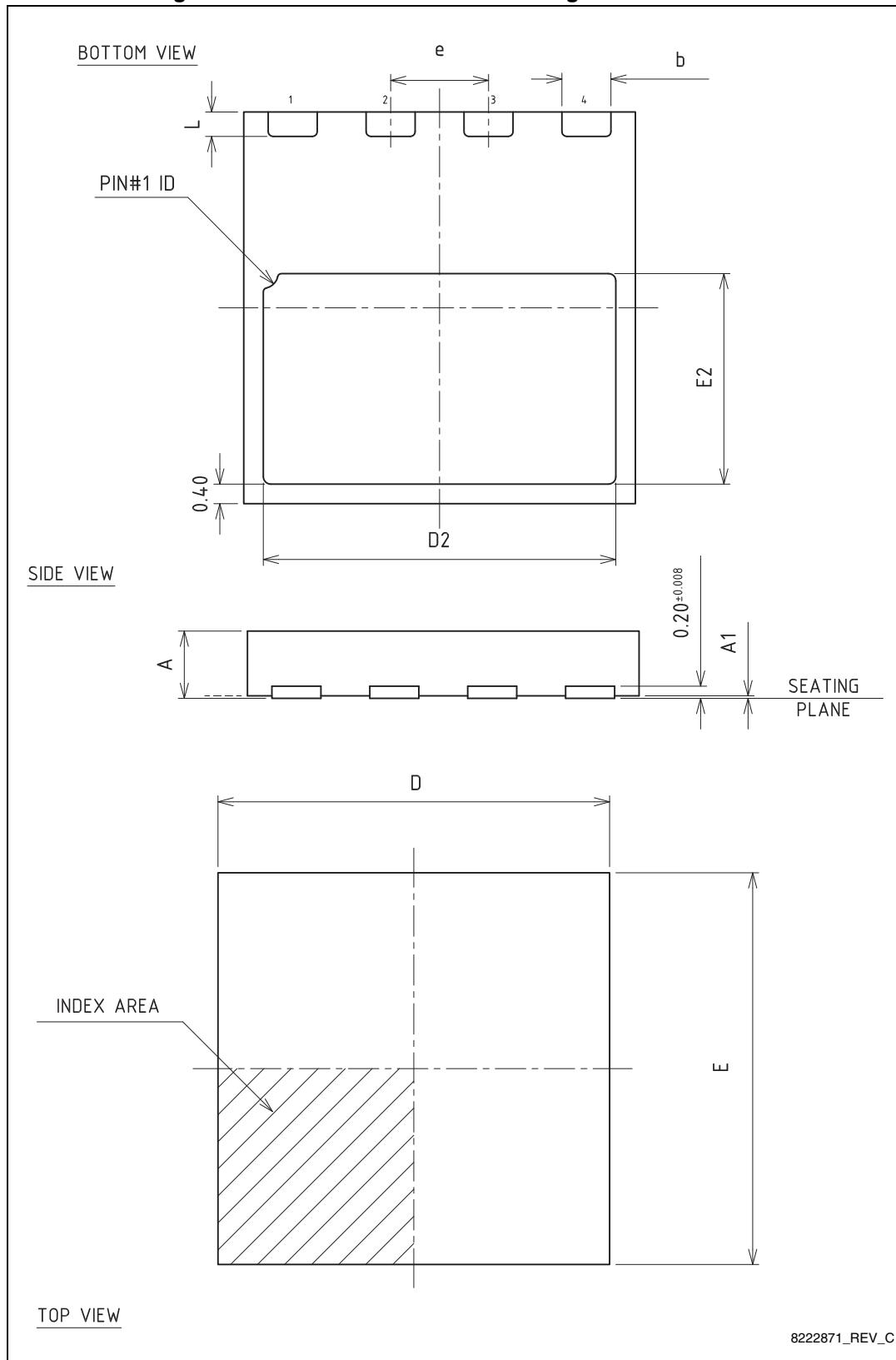
**Table 8. PowerFLAT™ 8x8 HV mechanical data**
