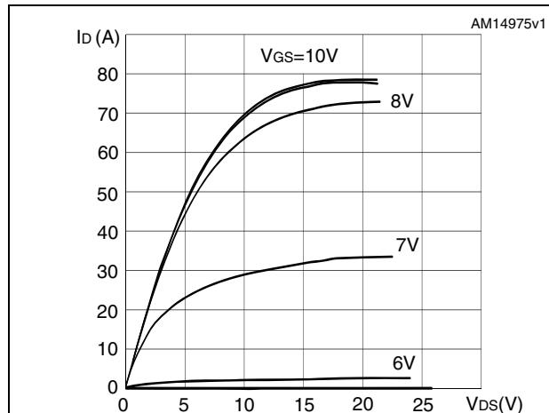
Figure 5. Transfer characteristics
