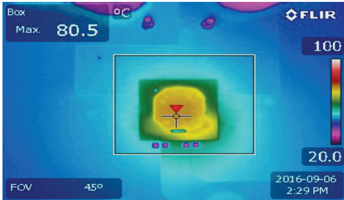
Figure 4. Thermal Image of LTM4636, V_{IN} = 12V , V_{OUT} = 1.0V , I_{LOAD} = 40A , Ambient Temperature = 23.0°C, No Forced Airflow
