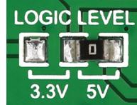
To switch between 3.3V or 5V power supplies, use the onboard zero-ohm SMD jumper. By default it's soldered in the 3.3V position.
