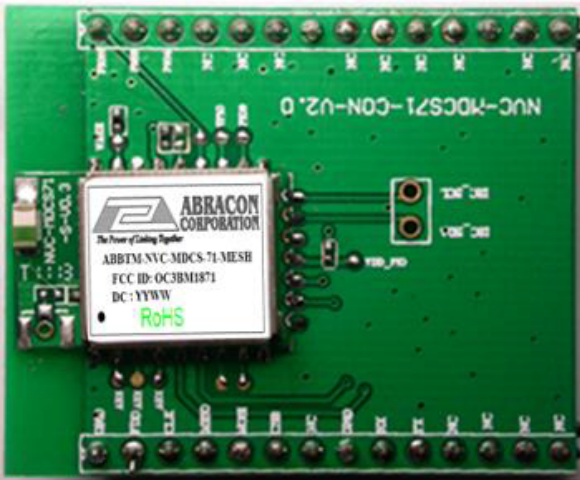
Figure 17: ABBTM-NVC-MDCS71-MESH-CON (41 x 33mm)
