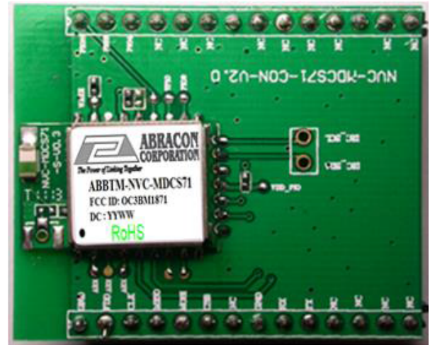
Figure 16: ABBTM-NVC-MDCS71-CON (41 x 33mm)
