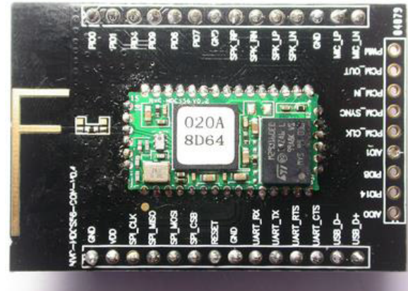
Figure 18: ABBTM-NVC-MDCS56-CON (49 x 33.5mm)
