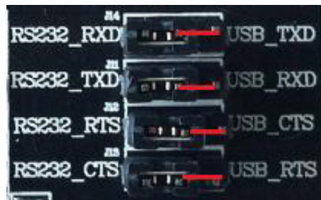
Figure 5: USB to serial jumper connect
