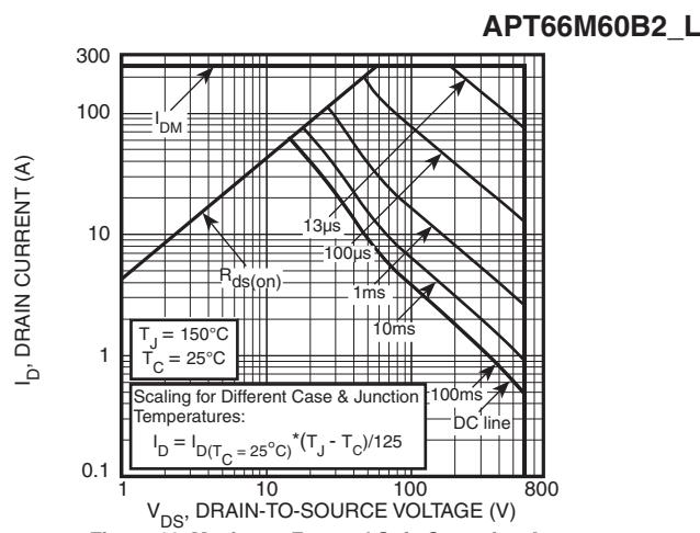
Figure 10, Maximum Forward Safe Operating Area
