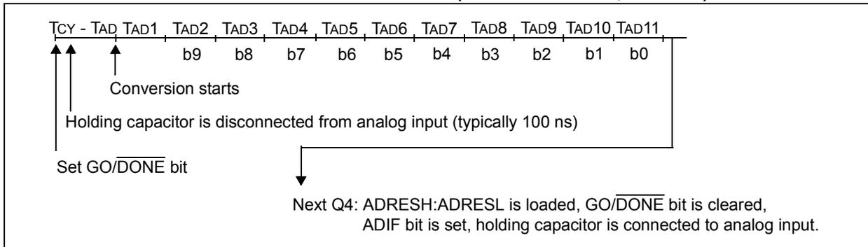
**FIGURE 21-4: A/D CONVERSION TAD CYCLES ( $\text{ACQT}<2:0> = 010, \text{TACQ} = 4 \text{ TAD}$ )**
