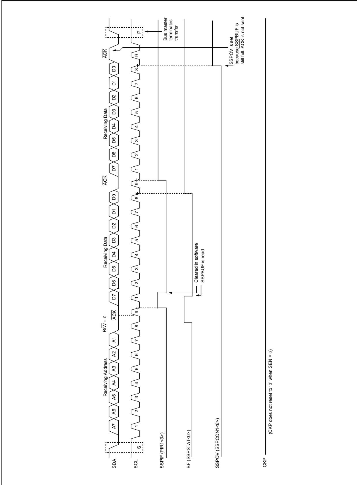
**FIGURE 18-9: I<sup>2</sup>C™ SLAVE MODE TIMING WITH SEN = 0 AND ADMSK<5:1> = 01011 (RECEPTION, 7-BIT ADDRESSING)**
