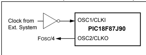
An external clock source may also be connected to the OSC1 pin in the HS mode, as shown in Figure 3-4. In this configuration, the divide-by-4 output on OSC2 is not available. Current consumption in this configuration will be somewhat higher than EC mode, as the internal oscillator's feedback circuitry will be enabled (in EC mode, the feedback circuit is disabled).
