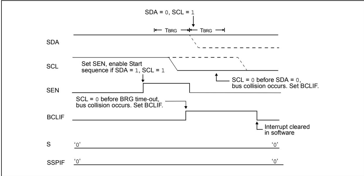
**FIGURE 18-30: BRG RESET DUE TO SDA ARBITRATION DURING START CONDITION**
