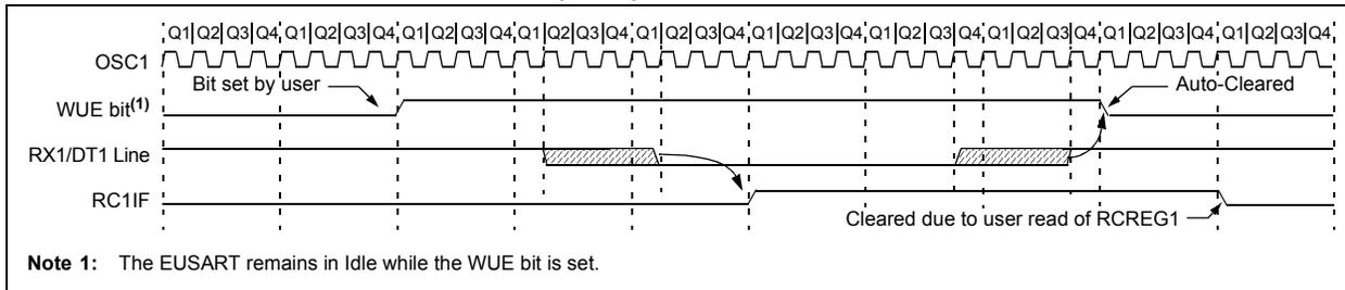
**FIGURE 19-9: AUTO-WAKE-UP BIT (WUE) TIMINGS DURING SLEEP**
