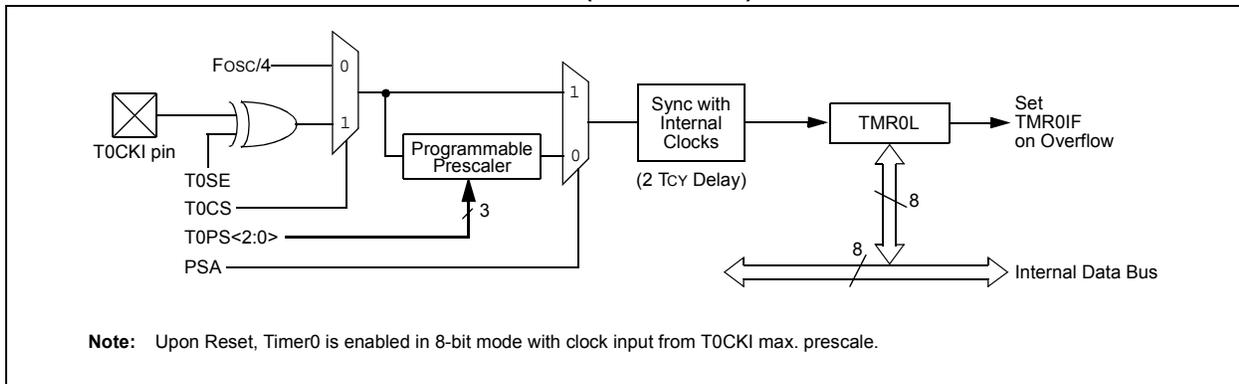
**FIGURE 11-2: TIMER0 BLOCK DIAGRAM (16-BIT MODE)**
