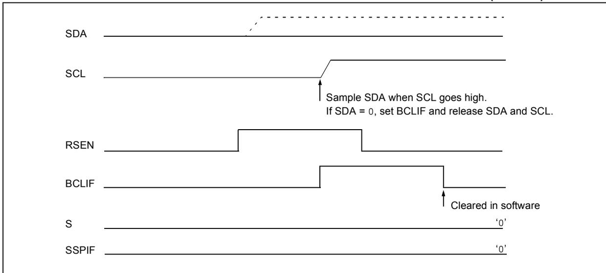
**FIGURE 18-32: BUS COLLISION DURING REPEATED START CONDITION (CASE 2)**
