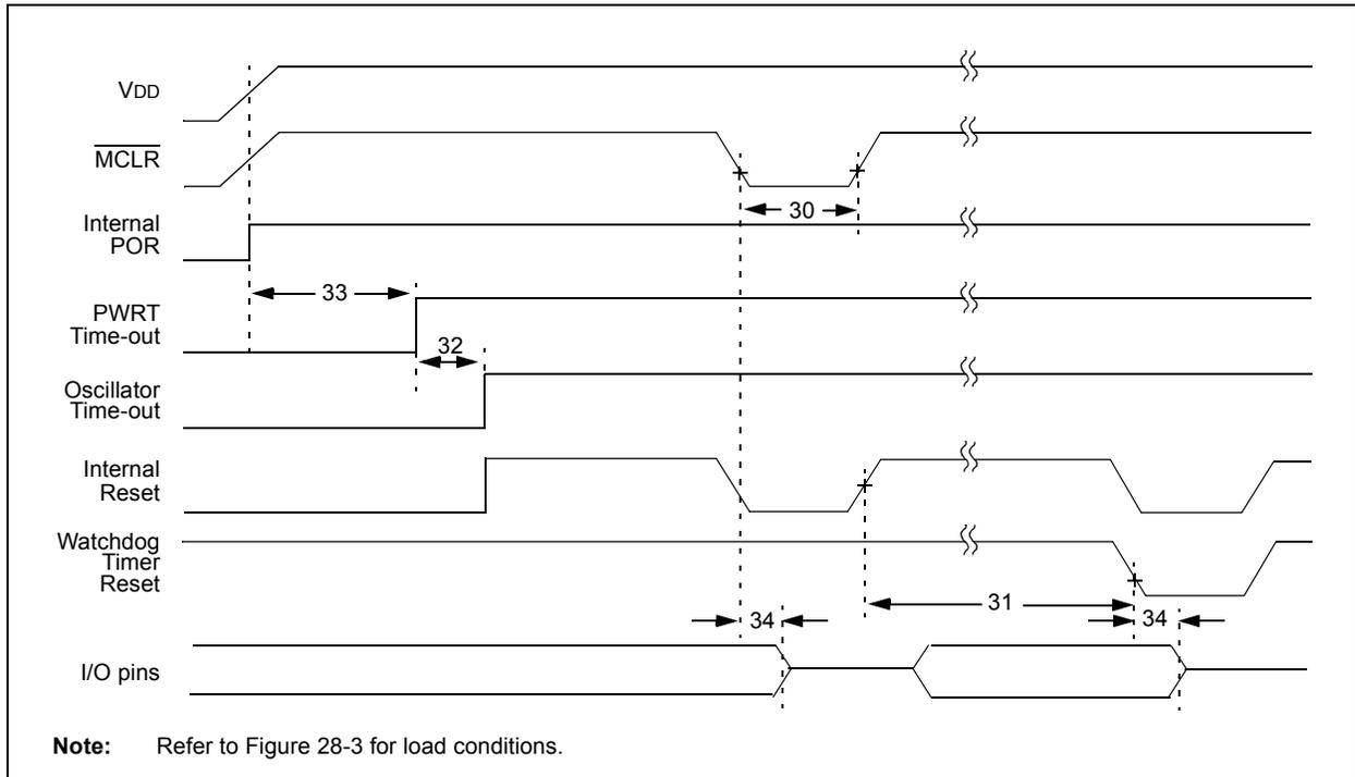
**TABLE 28-11: RESET, WATCHDOG TIMER, OSCILLATOR START-UP TIMER, POWER-UP TIMER AND BROWN-OUT RESET REQUIREMENTS**
