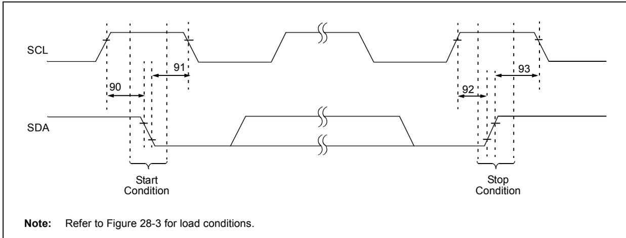
**TABLE 28-18: I<sup>2</sup>C™ BUS START/STOP BITS REQUIREMENTS (SLAVE MODE)**
