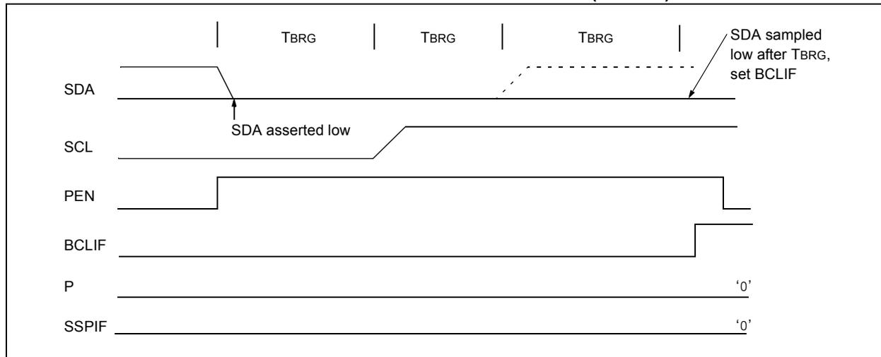
**FIGURE 18-34: BUS COLLISION DURING A STOP CONDITION (CASE 2)**
