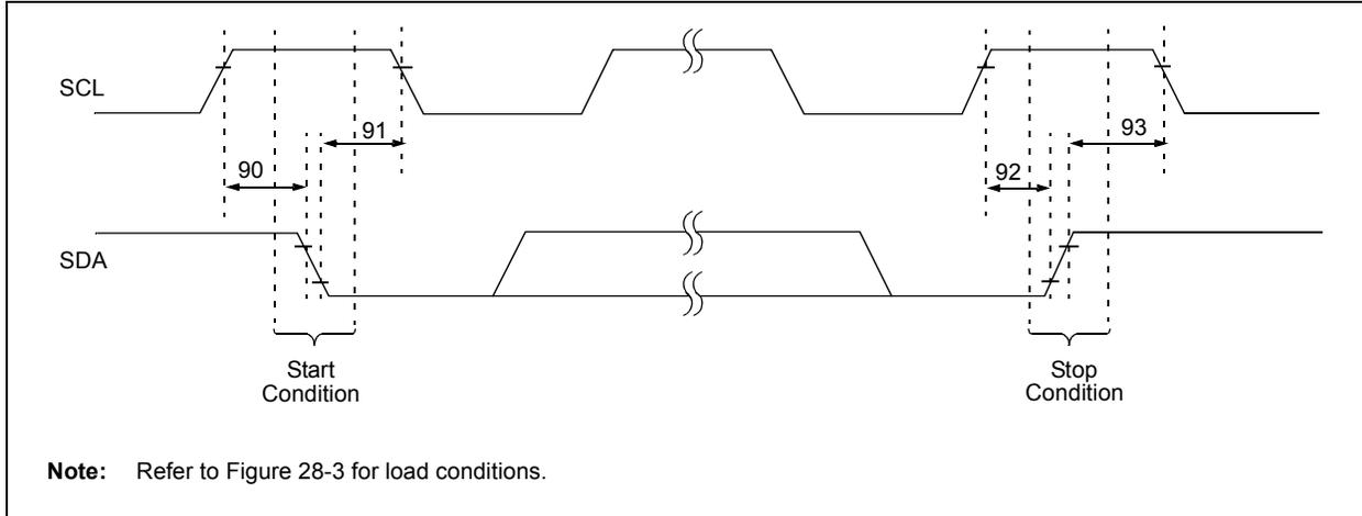
**TABLE 28-20: MSSP I<sup>2</sup>C™ BUS START/STOP BITS REQUIREMENTS**
