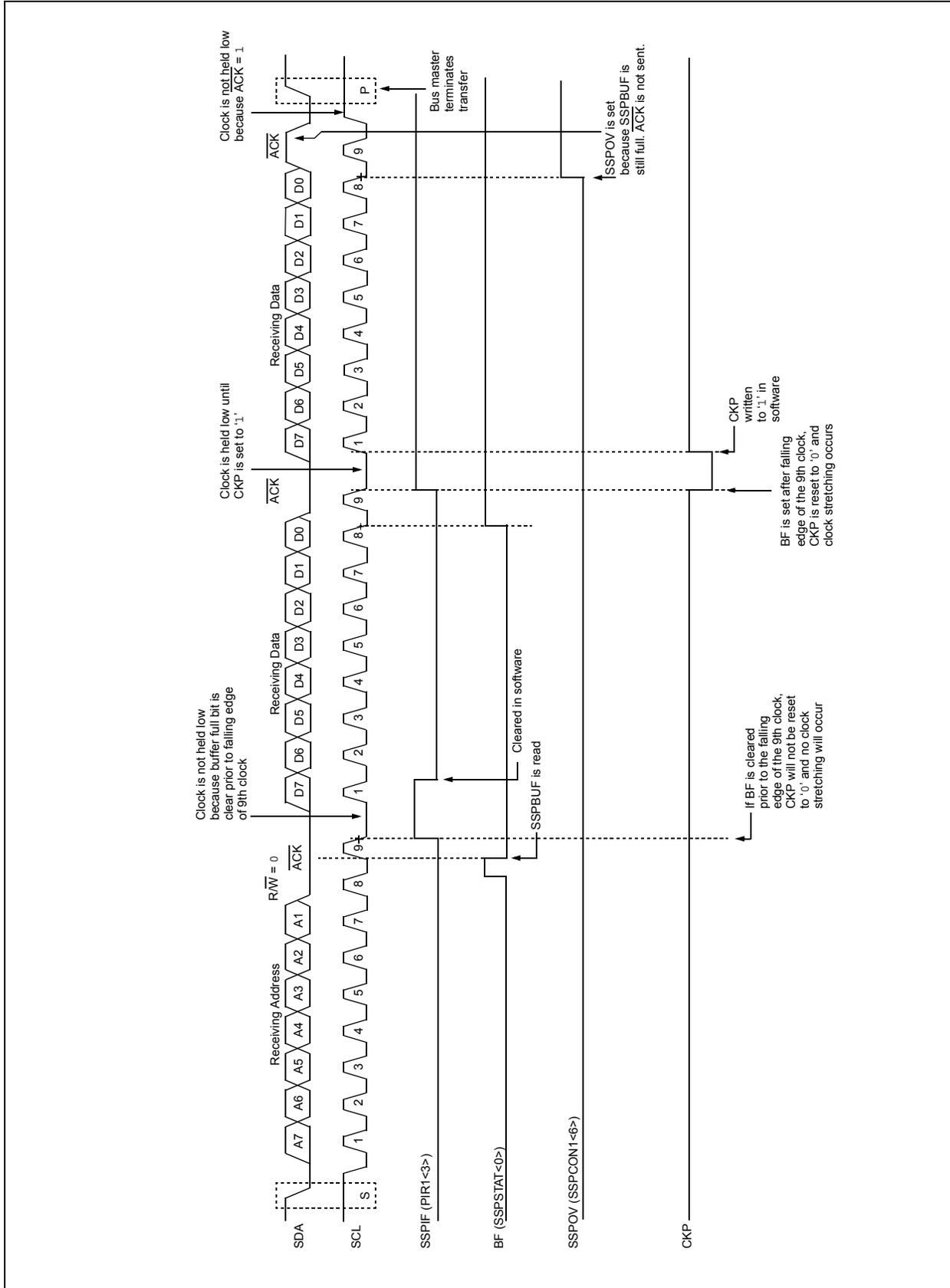
**FIGURE 18-16: I<sup>2</sup>C™ SLAVE MODE TIMING WITH SEN = 1 (RECEPTION, 10-BIT ADDRESSING)**
