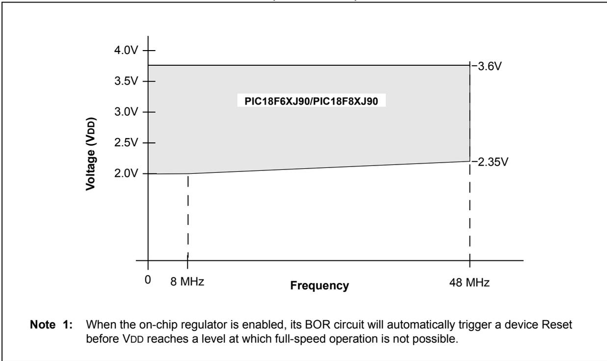
**FIGURE 28-2: VOLTAGE-FREQUENCY GRAPH, REGULATOR DISABLED (INDUSTRIAL)<sup>(1,2)</sup>**
