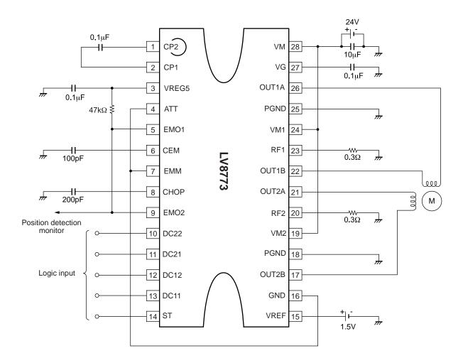
The formulae for setting the constants in the examples of the application circuits above are as follows: Constant current (100%) setting
