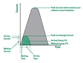
Figure 11 – Arcing and melting currents plus arcing, melting and clearing
