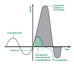
Figure 13 - Current-limiting Fuse
