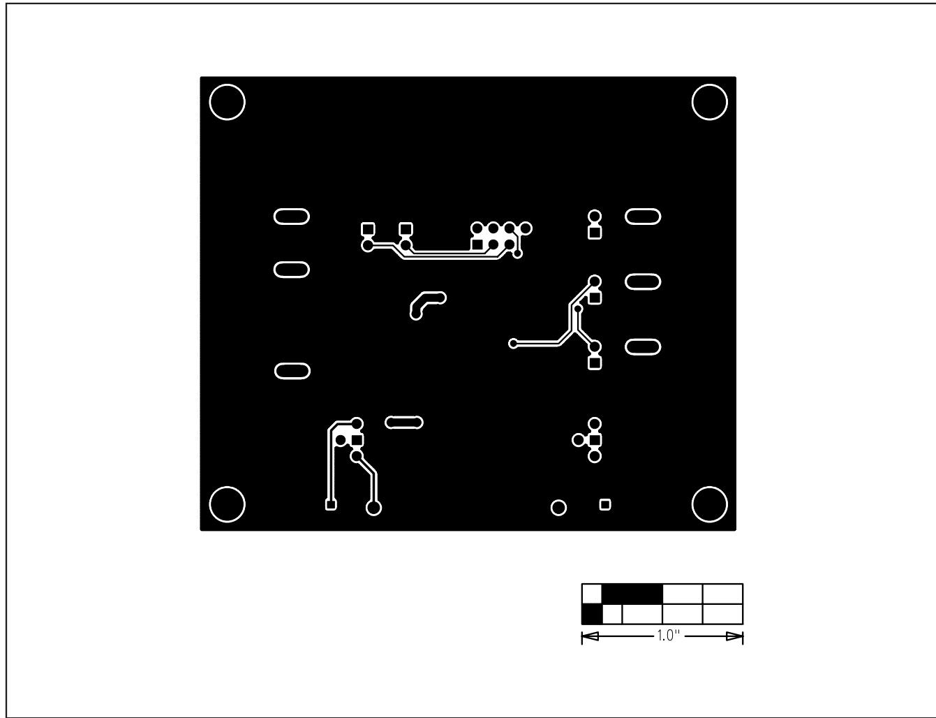
Figure 4. MAX9921 EV Kit PCB Layout—Solder Side
