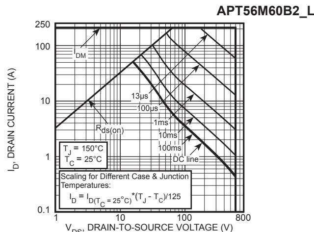
Figure 10, Maximum Forward Safe Operating Area
