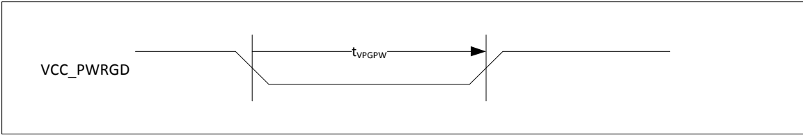
FIGURE 43-1: VCC_PWRGD TIMING DIAGRAM
