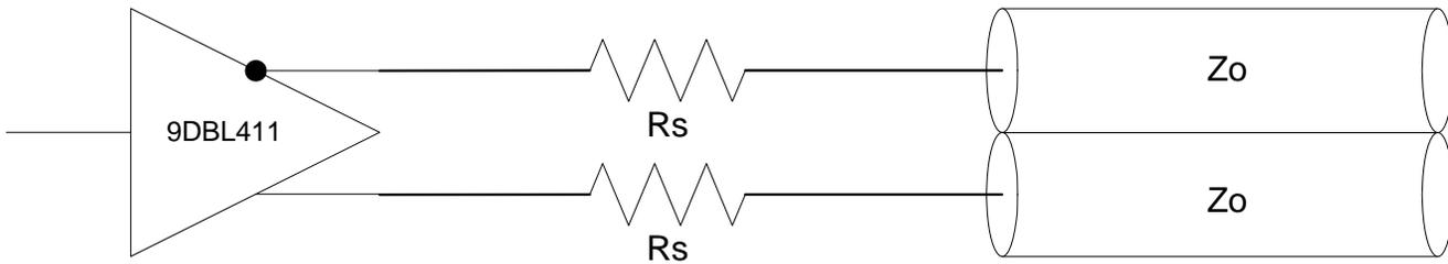
$Z_o - 17 = R_s$  (ohms), where  $Z_o$  is the single-ended intrinsic impedance of the board transmission line. Single-ended intrinsic impedance is  $\frac{1}{2}$  that of the differential impedance.
