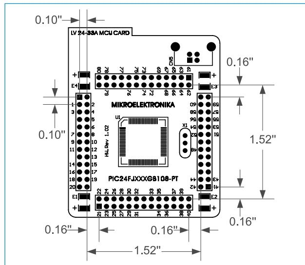
Figure 48: Dimensions of MCU card for *MCU Card 16*
