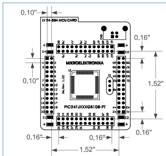
Figure 42: Dimensions of MCU card for *MCU Card 14*
