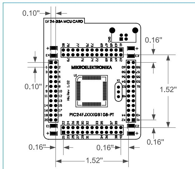
Figure 45: Dimensions of MCU card for *MCU Card 15*
