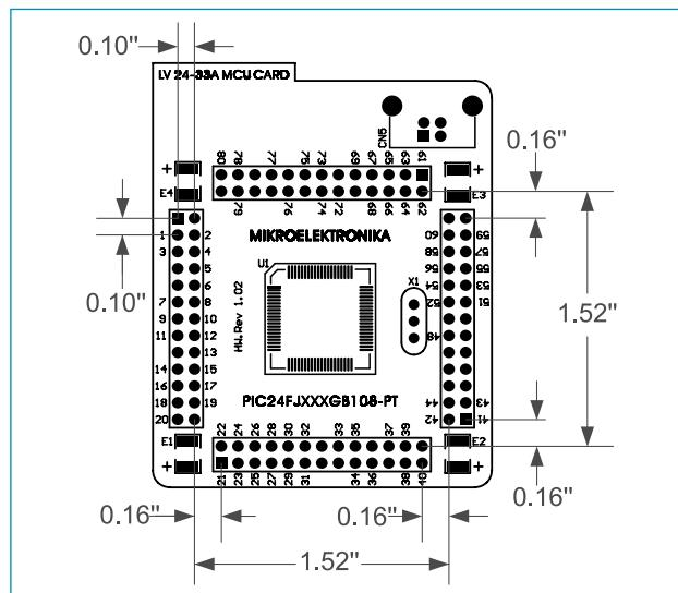
Figure 39: Dimensions of MCU card for MCU Card 13
