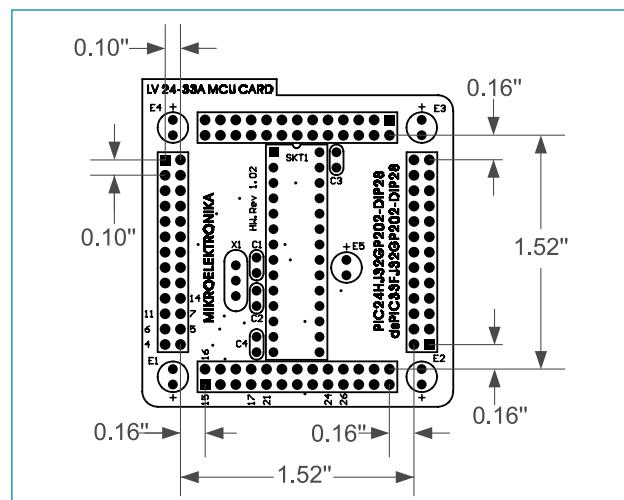
Figure 33: Dimensions of MCU card for *MCU Card 11*
