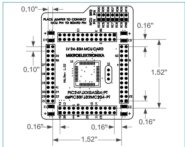
Figure 36: Dimensions of MCU card for *MCU Card 12*
