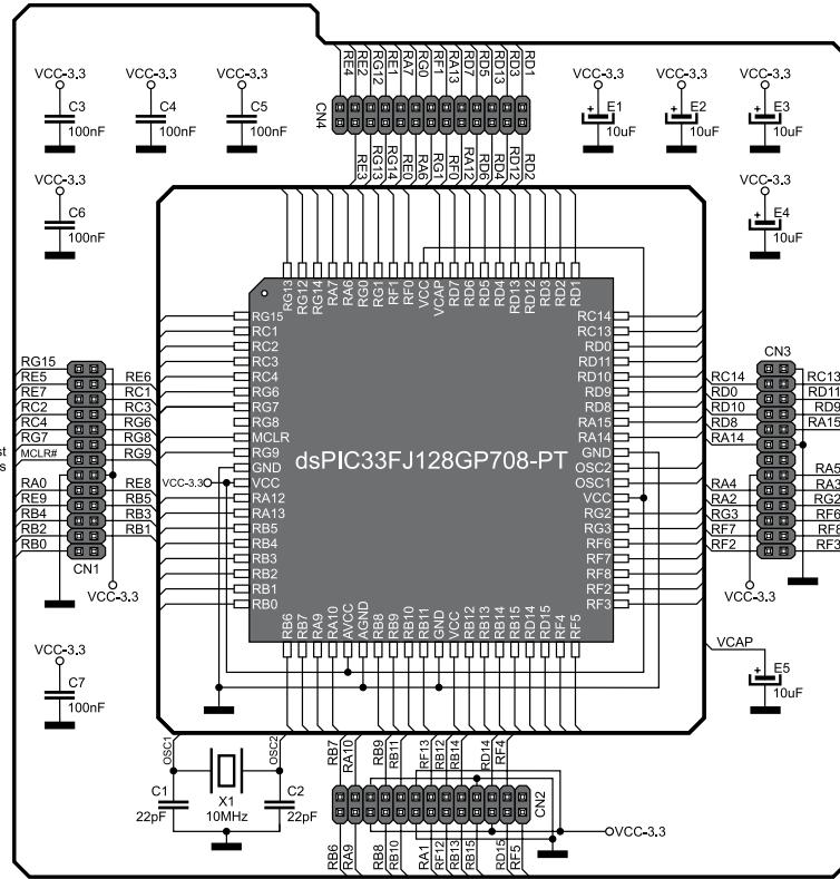
Figure 10: 80-pin MCU card *MCU Card 4* and microcontroller connection schematic
