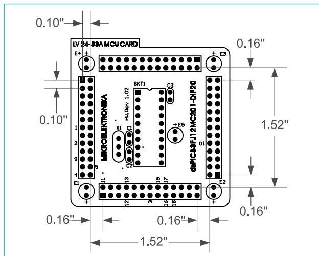
Figure 30: Dimensions of MCU card for *MCU Card 10*
