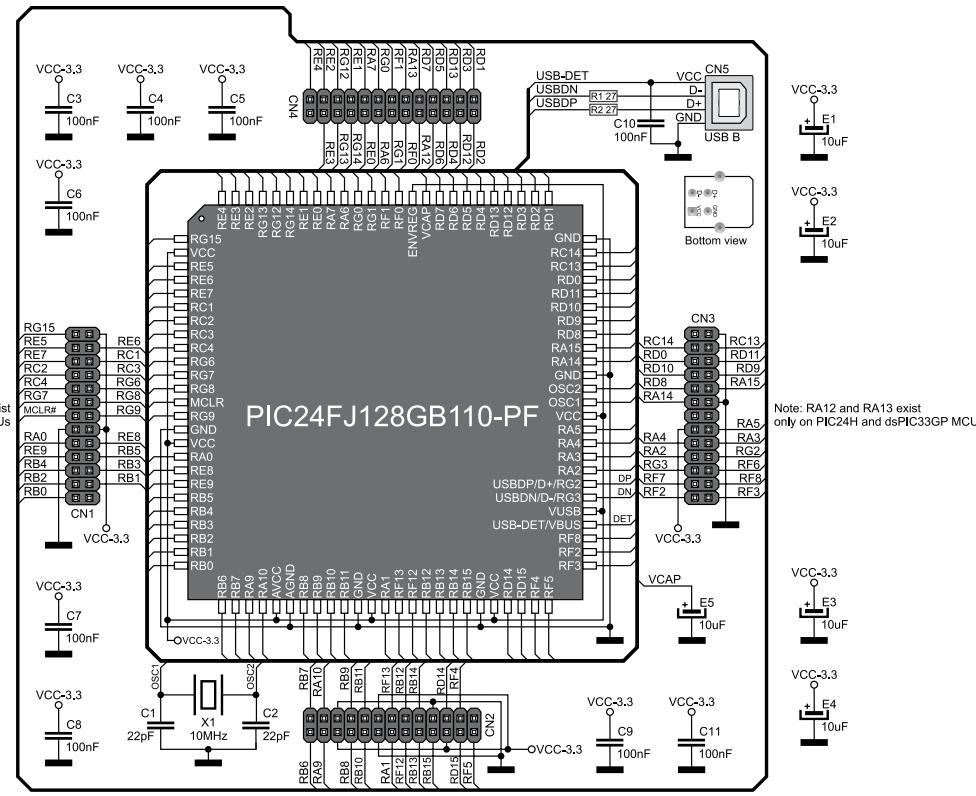
Figure 46: 100-pin MCU card *MCU Card 16* and microcontroller connection schematic
