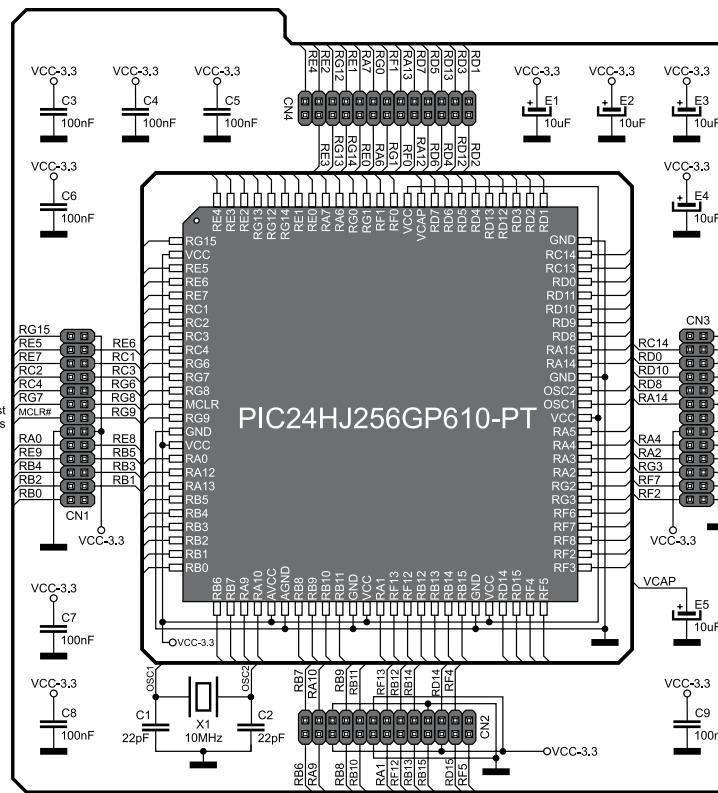
Figure 16: 100-pin MCU card *MCU Card 6* and microcontroller connection schematic
