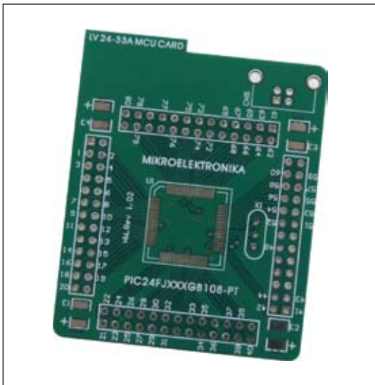
Figure 41: Empty MCU card MCU Card 14
