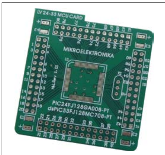
Figure 8: Empty MCU card MCU Card 3
