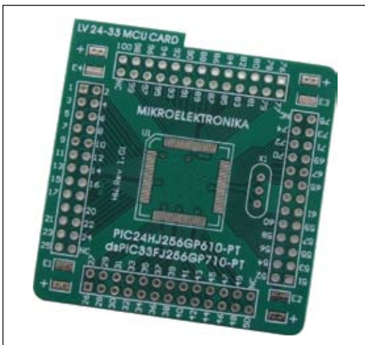
Figure 17: Empty MCU card MCU Card 6
