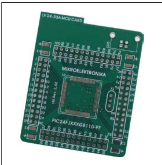
Figure 47: Empty MCU card MCU Card 16
