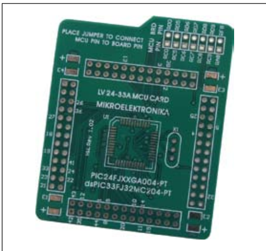
Figure 35: Empty MCU card MCU Card 12
