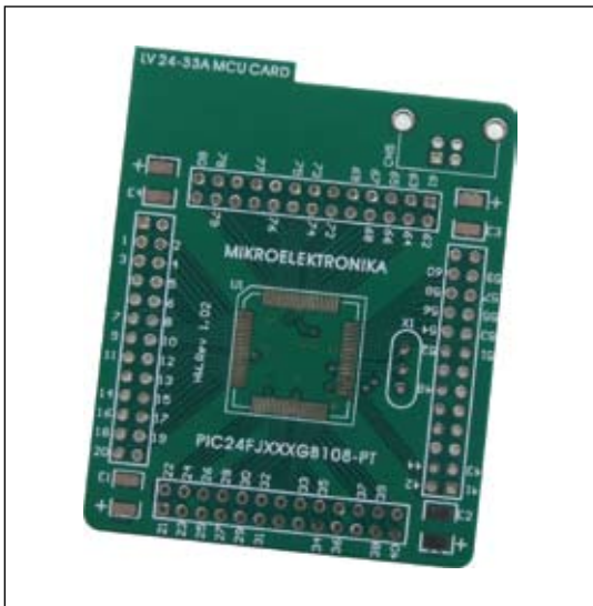
Figure 41: Empty MCU card MCU Card 14
