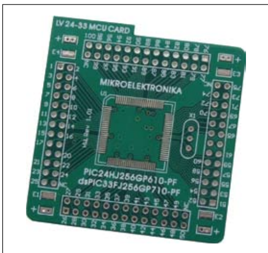
Figure 23: Empty MCU card MCU Card 8
