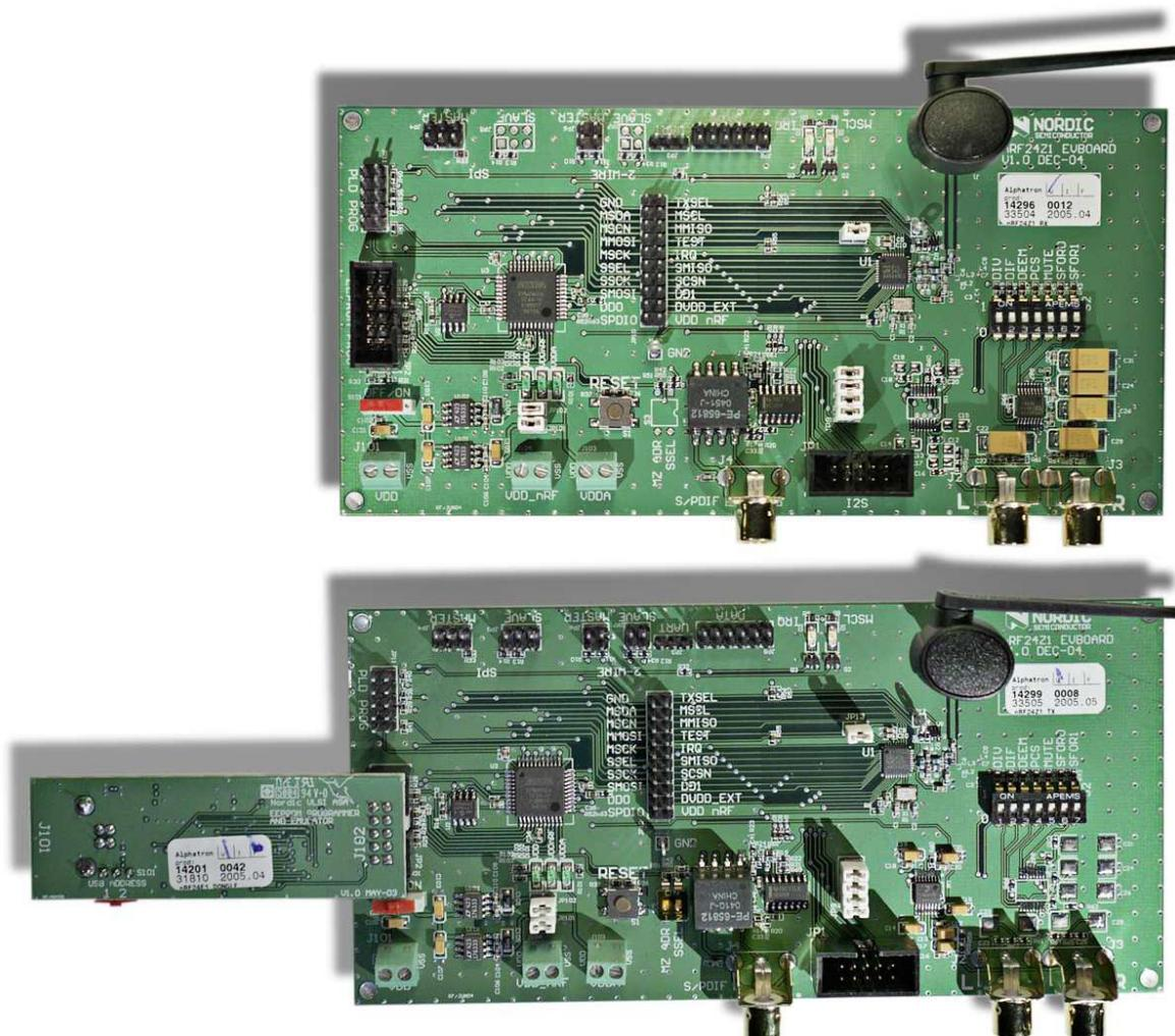
Figure 1: The **nRF24Z1-EVBOARD**
