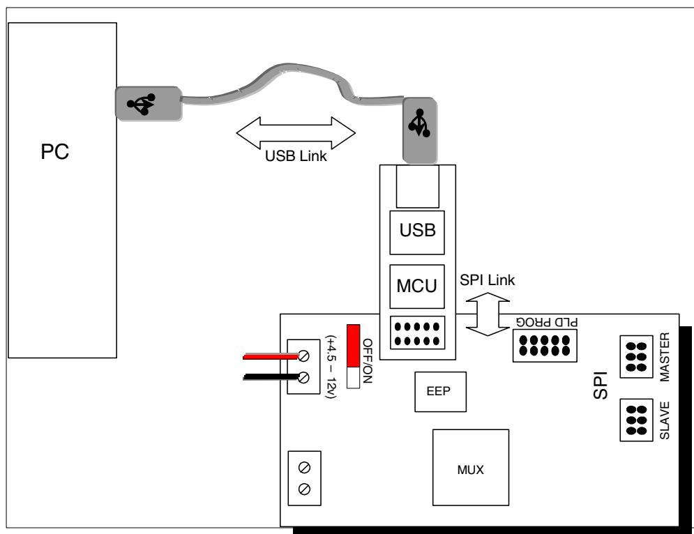
Figure 2: **nRF24Z1-EVBOARD** with programming dongle
