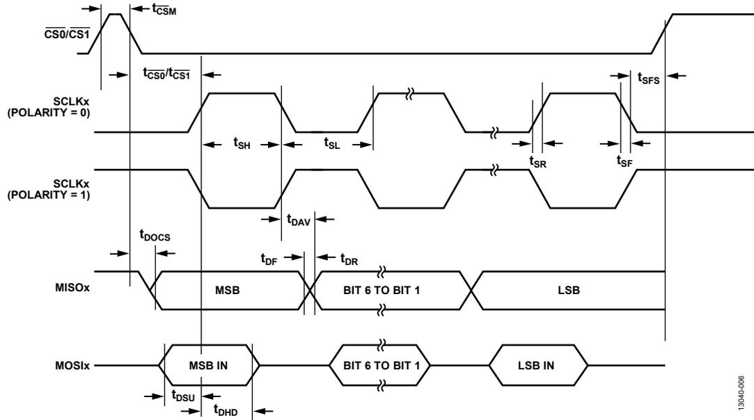
Figure 6. SPI Slave Mode Timing (Phase Mode = 0)
