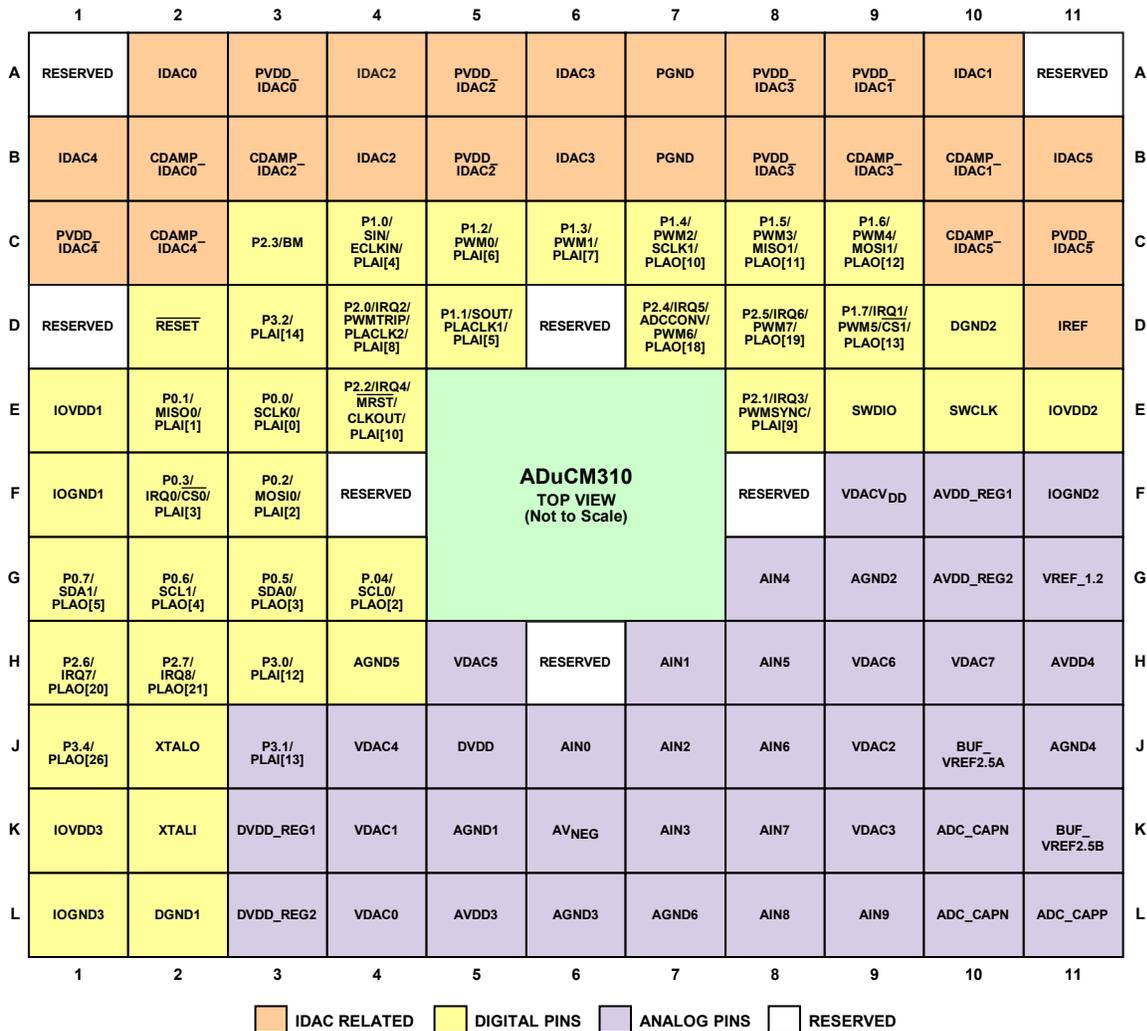
Figure 7. Pin Configuration
