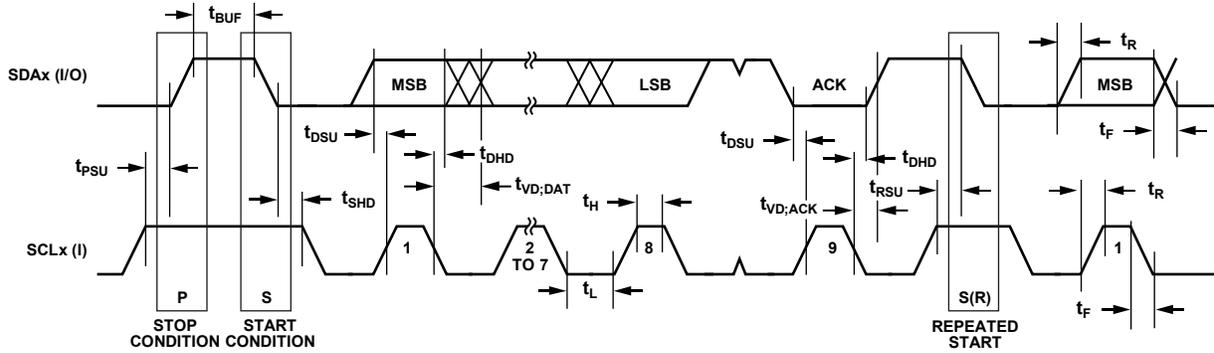
Figure 2. I<sup>2</sup>C Compatible Interface Timing
