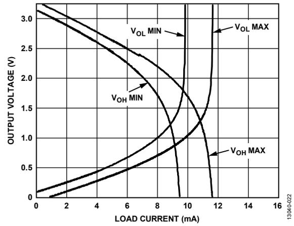
Figure 22. Typical Output Voltage vs. Load Current
