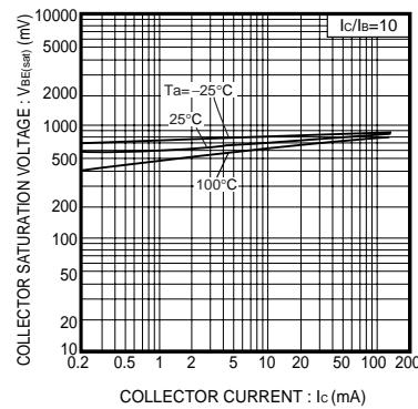
Fig.9 Base-emitter saturation voltage vs. collector current (II)
