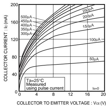
Fig.2 Grounded emitter output characteristics ( II )
