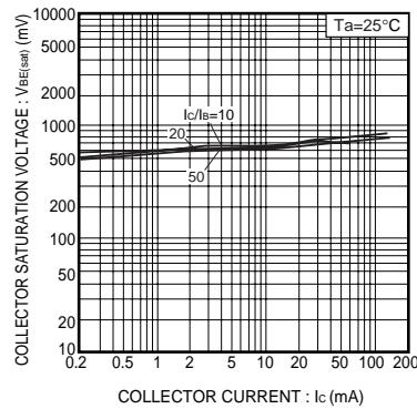
Fig.8 Base-emitter saturation voltage vs. collector current (I)
