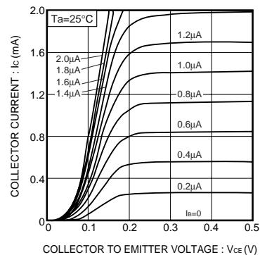
Fig.1 Grounded emitter output characteristics ( I )
