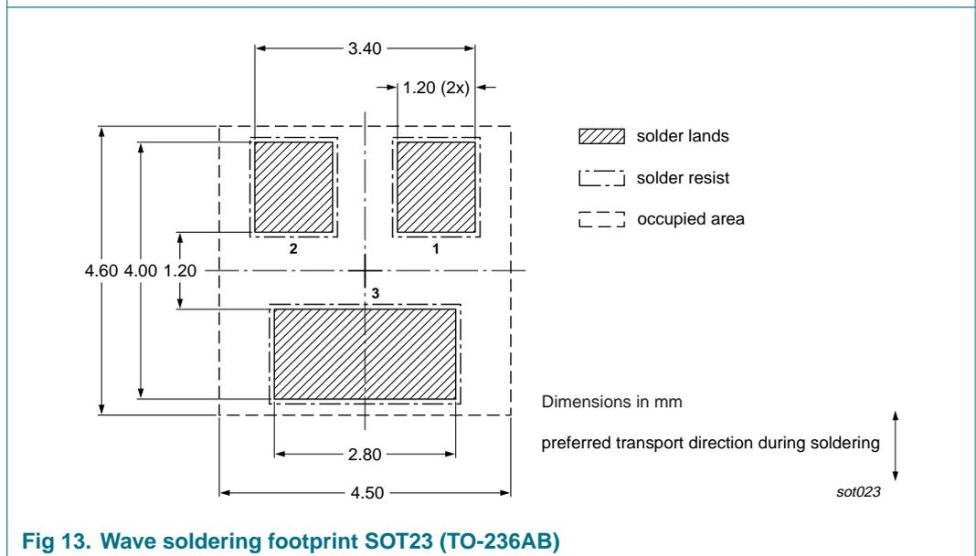
**Fig 13. Wave soldering footprint SOT23 (TO-236AB)**
