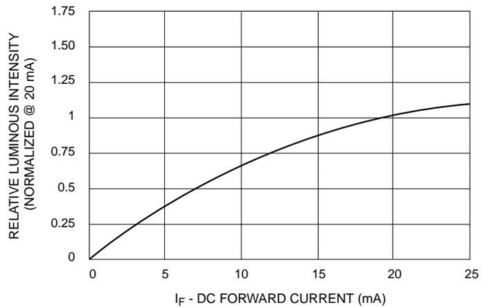
**Fig.2 Relative Luminous Intensity vs. DC Forward Current**
