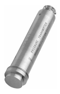
The BL pressure transmitter has a conventional 4 mA to 20 mA output and is available with accuracies to 0.25%. The BL is approved for Factory Mutual as an intrinsically safe\* device for use in hazardous areas. Rated for Class 1, Div. 1 groups A through G.
