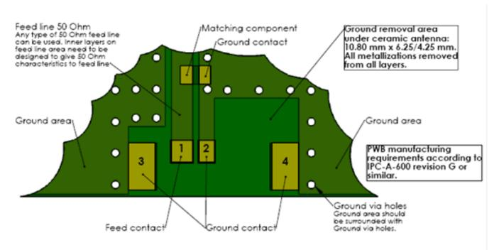
Note: Electrical characteristics are measured on test pwb with matching circuit (2.2 nH shunt matching inductor on feed).
