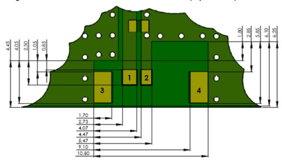
Recommended ground clearance area under antenna on PWB (bottom surface)
