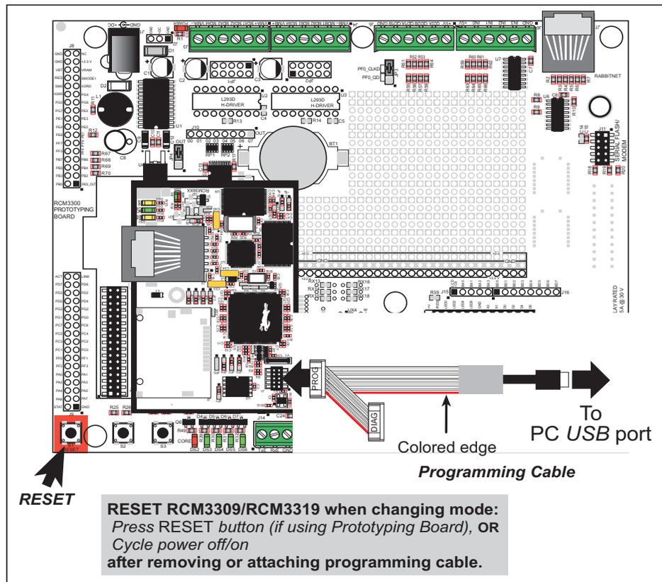
**Figure 9. Switching Between Program Mode and Run Mode**
