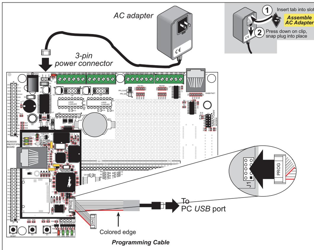
**Figure 3. Connect Programming Cable and Power Supply**
