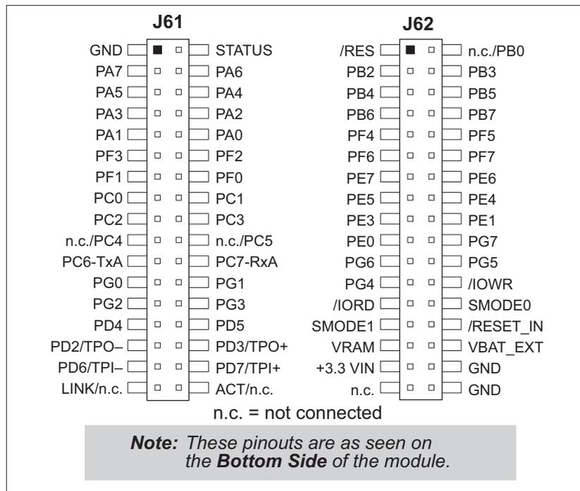
**Figure 5. RCM3309/RCM3319 Pinouts**
