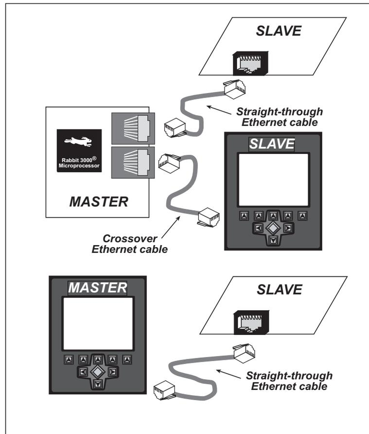
Figure 1. Connecting Peripheral Cards to a Master
