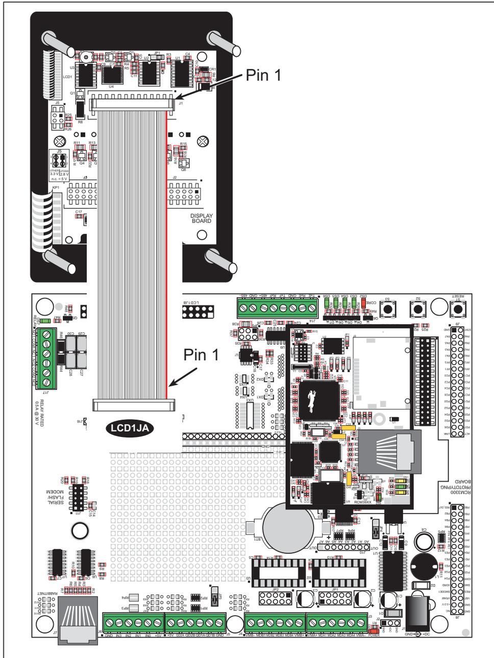
**Figure C-10. Connecting LCD/Keypad Module to Prototyping Board**
