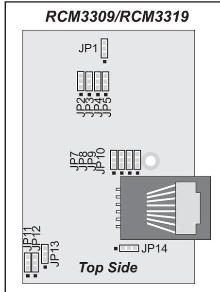
**Figure A-5. Location of RCM3309/RCM3319 Configurable Positions**
