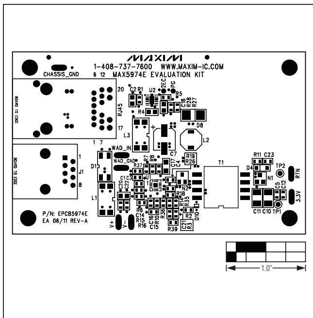
Figure 2. MAX5974E EV Kit Component Placement Guide—Component Side
