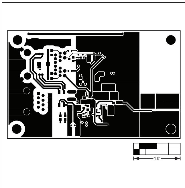
Figure 6. MAX5974E EV Kit PCB Layout—Solder Side
