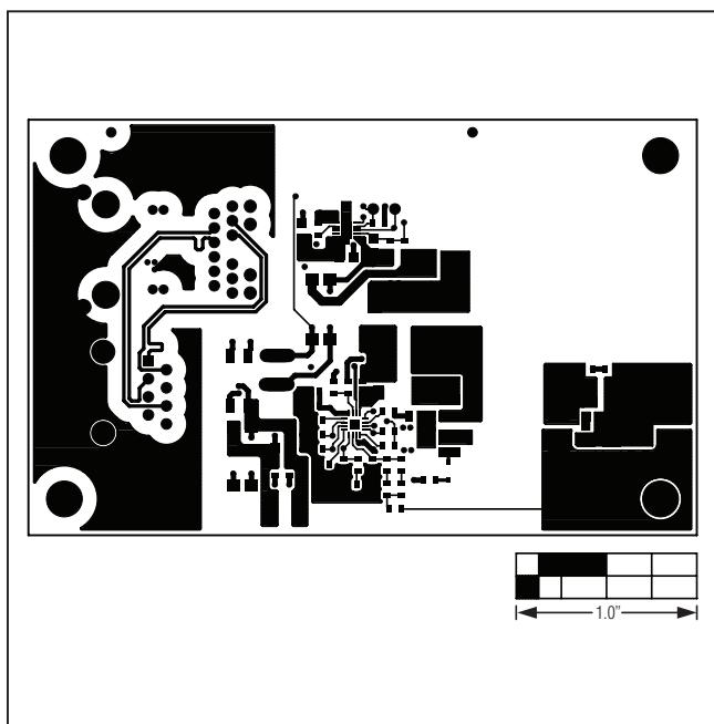
Figure 3. MAX5974E EV Kit PCB Layout—Component Side
