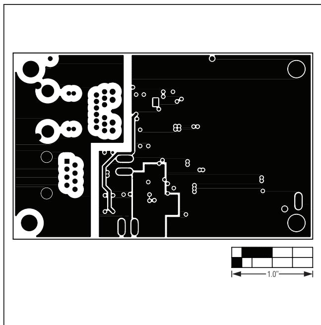
Figure 4. MAX5974E EV Kit PCB Layout—GND Layer 2
