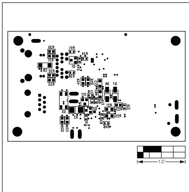
Figure 7. MAX5974E EV Kit Component Placement Guide—
