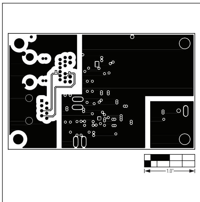
Figure 5. MAX5974E EV Kit PCB Layout—Signal Layer 3
