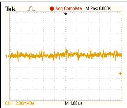
Figure 4. Noise at  $V_{OUT} = 12V$ ,  $I_{OUT} = 0mA$ .
