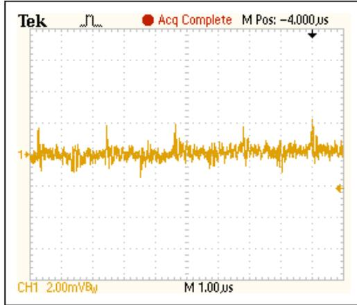
Figure 7. Noise at  $V_{OUT} = 15V$ ,  $I_{OUT} = 40mA$ .
