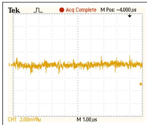
Figure 5. Noise at  $V_{OUT} = 15V$ ,  $I_{OUT} = 0mA$ .
