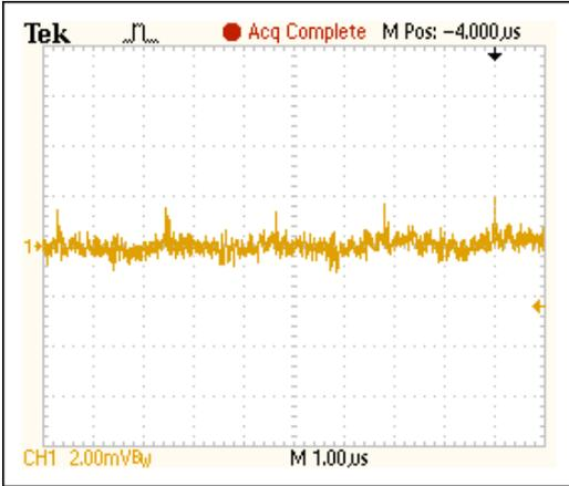
Figure 6. Noise at  $V_{OUT} = 12V$ ,  $I_{OUT} = 90mA$ .
