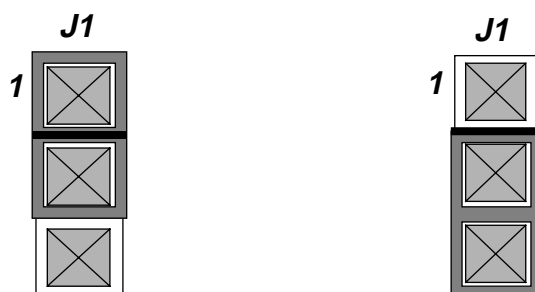
FIGURE 2-3 Power-On Reset Source Selection
