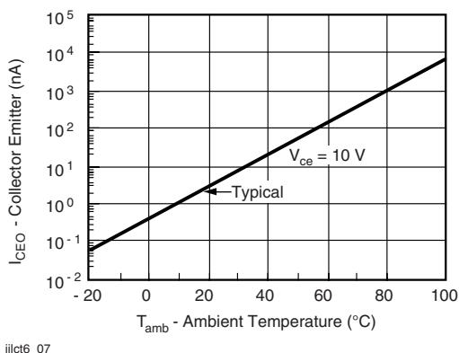
Fig. 7 - Collector Emitter Leakage Current vs. Temperature
