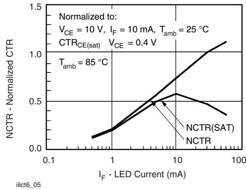
Fig. 5 - Normalized Non-Saturated and Saturated CTR vs.
