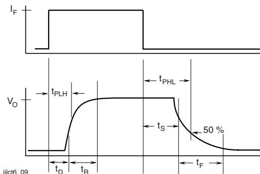
Fig. 9 - Switching Timing
