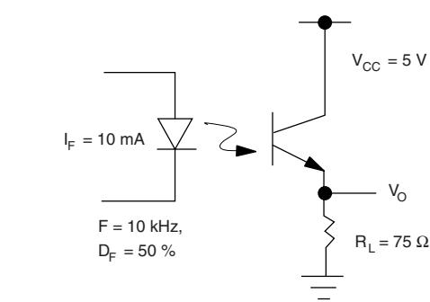
Fig. 10 - Switching Schematic
