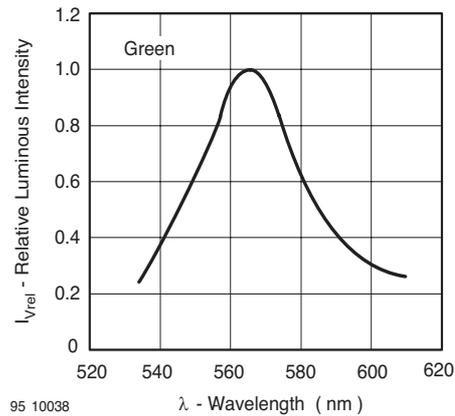
Figure 20. Relative Intensity vs. Wavelength
