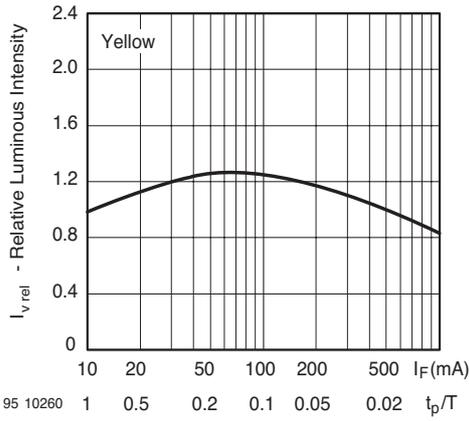
Figure 13. Rel. Lumin. Intensity vs. Forw. Current/Duty Cycle
