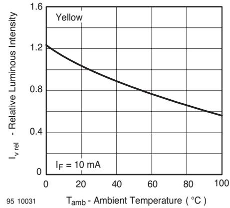
Figure 12. Rel. Luminous Intensity vs. Ambient Temperature
