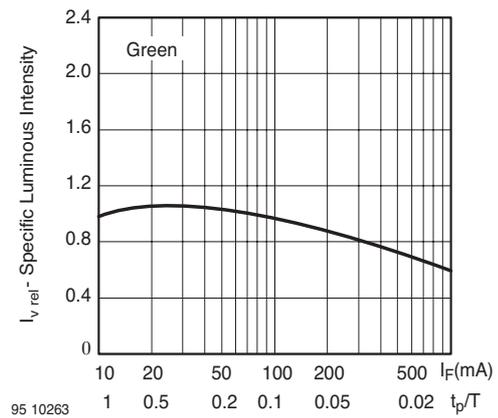
Figure 18. Specific Luminous Intensity vs. Forward Current
