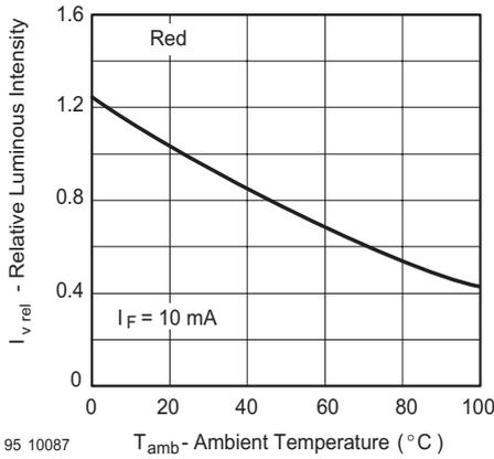
Figure 7. Rel. Luminous Intensity vs. Ambient Temperature
