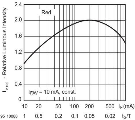
Figure 8. Rel. Lumin. Intensity vs. Forw. Current/Duty Cycle
