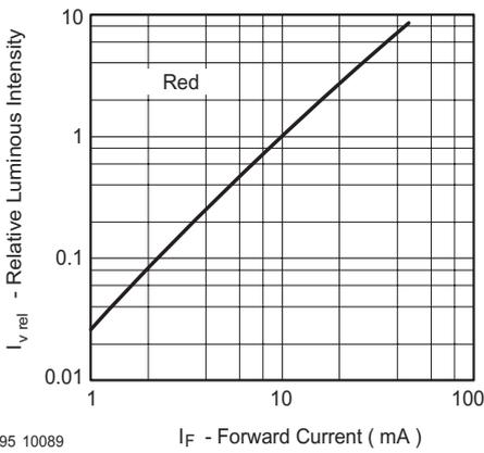
Figure 9. Relative Luminous Intensity vs. Forward Current
