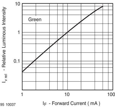
Figure 19. Relative Luminous Intensity vs. Forward Current
