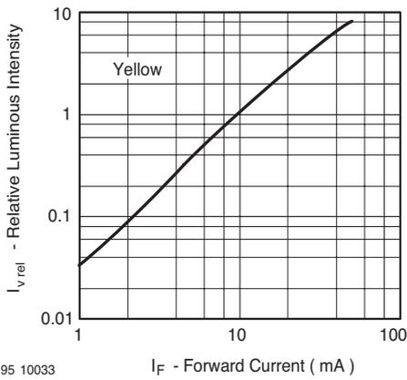
Figure 14. Relative Luminous Intensity vs. Forward Current
