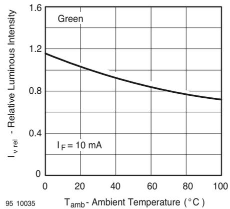
Figure 17. Rel. Luminous Intensity vs. Ambient Temperature
