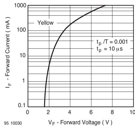
Figure 11. Forward Current vs. Forward Voltage
