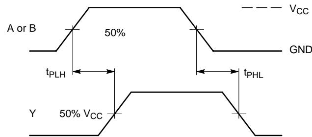
Figure 3. Switching Waveforms
