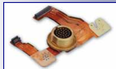
Flex Termination with MIL-C-26482 Special Connector
