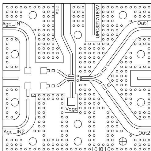
**EVALUATION BOARD ASSEMBLY****INTERNAL BLOCK DIAGRAM**
