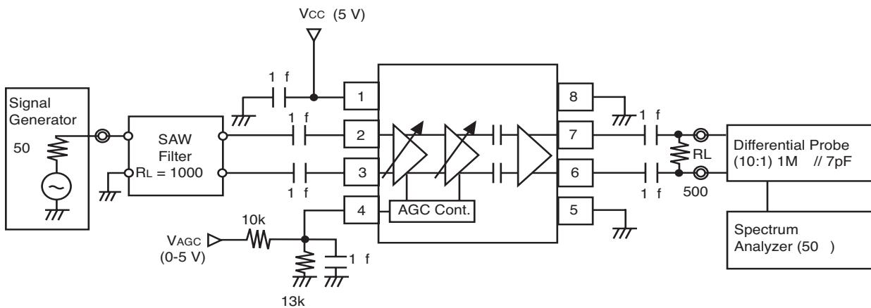
EVALUATION BOARD SCHEMATIC AND TEST
