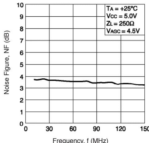
\* VAGC shown as applied in the evaluation circuit (see page 5) through a resistive bridge (voltage divider). Actual voltage range on the pin of the IC is 0 to 3 V.
