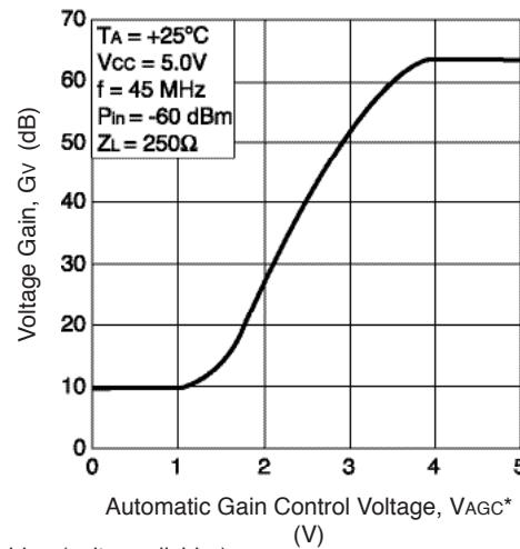
\* VAGC shown as applied in the evaluation circuit (see page 5) through a resistive bridge (voltage divider). Actual voltage range on the pin of the IC is 0 to 3 V.
