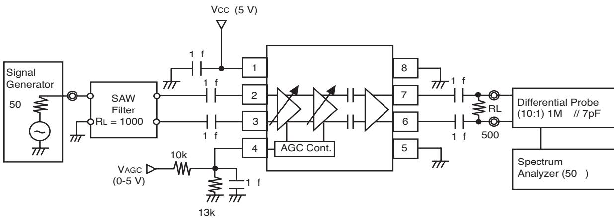
EVALUATION BOARD SCHEMATIC AND TEST
