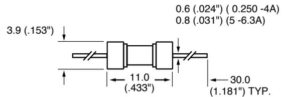
Axial Lead Material: Solder coated copper.
