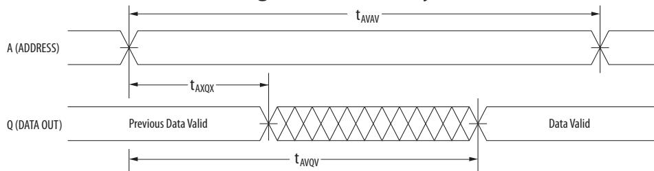
**Figure 3.3B Read Cycle 2**
