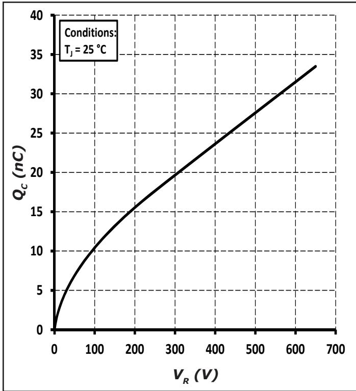
Figure 5. Total Capacitance Charge vs. Reverse Voltage
