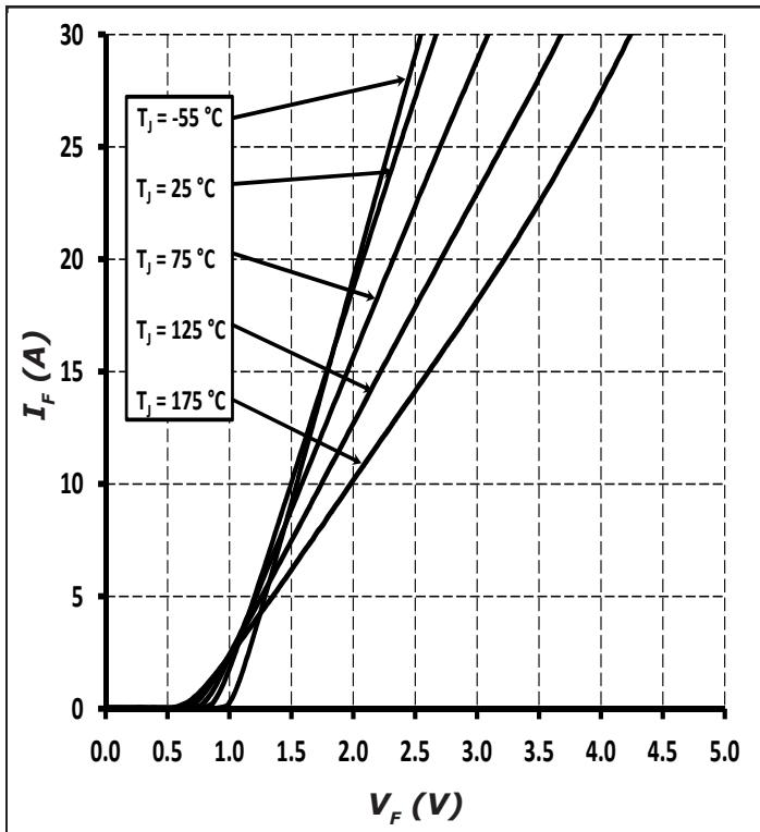
Figure 1. Forward Characteristics
