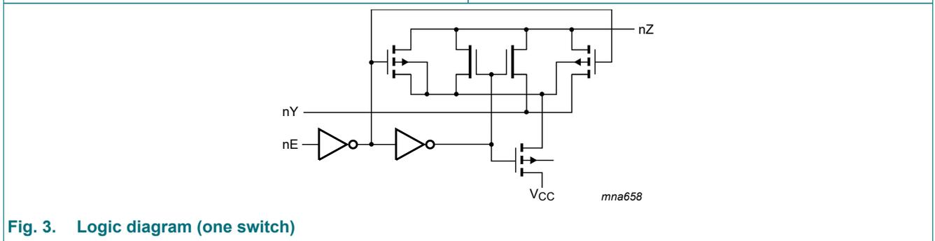
Fig. 3. Logic diagram (one switch)
