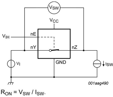
Fig. 8. Test circuit for measuring ON resistance
