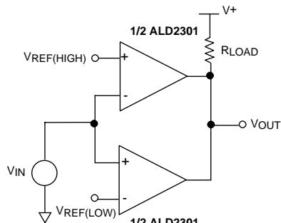
MINIMUM  $R_{LOAD} = 1.5\text{ k}\Omega$
