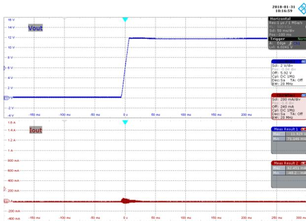
**Figure 50** – 230 VAC 60 Hz, No-Load Start-up.
