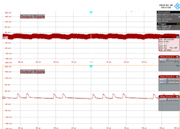
Figure 112 – 90 VAC 47 Hz, 25% Load. CH1: V_{OUT} , 40 mV / div., 10 ms / div. Zoom: 20 \mu s / div. Voltage Ripple ( V_{OUT(PK-PK)} ) = 50.5 mV).
