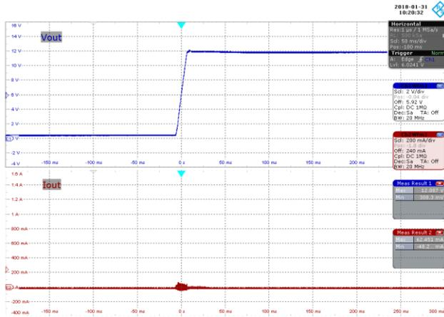
**Figure 56** – 90 VAC 60 Hz, No-Load Start-up.
