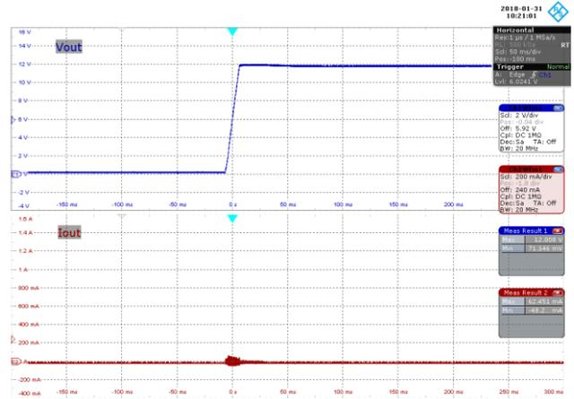
**Figure 57** – 115 VAC 60 Hz, No-Load Start-up.
