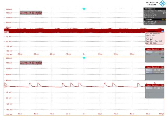
**Figure 113** – 115 VAC 47 Hz, 25% Load.
