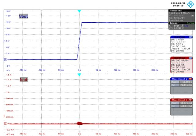
**Figure 49** – 115 VAC 60 Hz, No-Load Start-up.
