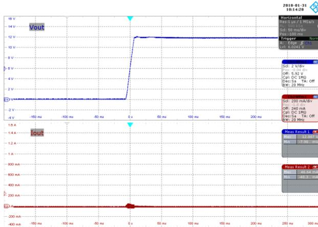
**Figure 48** – 90 VAC 60 Hz, No-Load Start-up.
