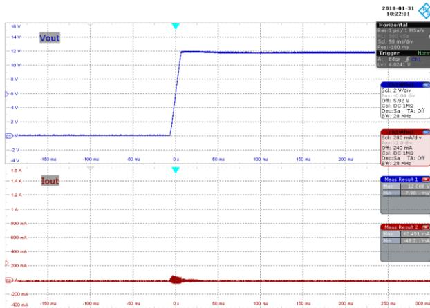
**Figure 58** – 230 VAC 60 Hz, No-Load Start-up.
