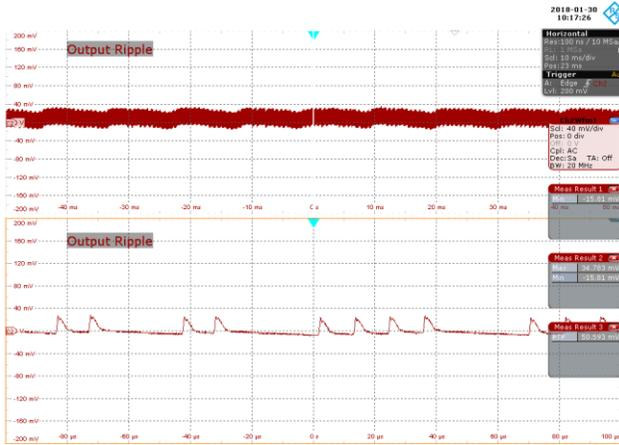
**Figure 112** – 90 VAC 47 Hz, 25% Load.
