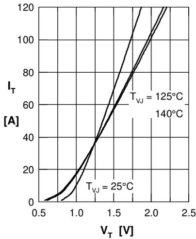
Fig. 1 Forward characteristics
