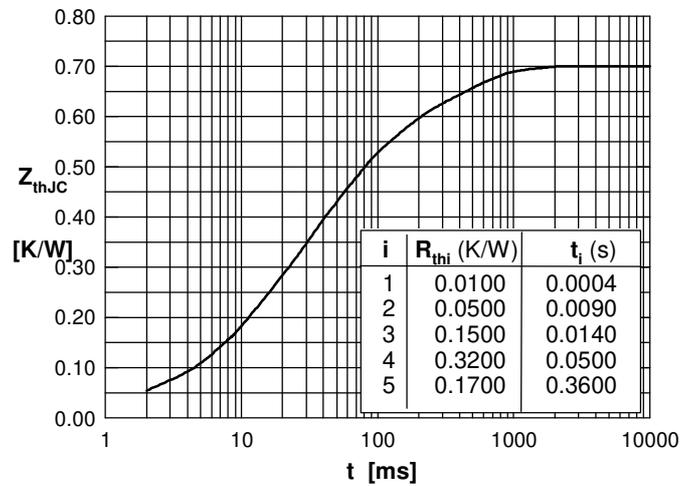
Fig. 8 Transient thermal impedance junction to case
