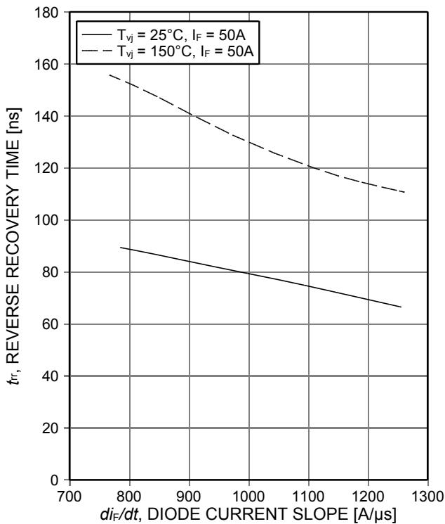
Figure 19. Typical reverse recovery time as a function of diode current slope
