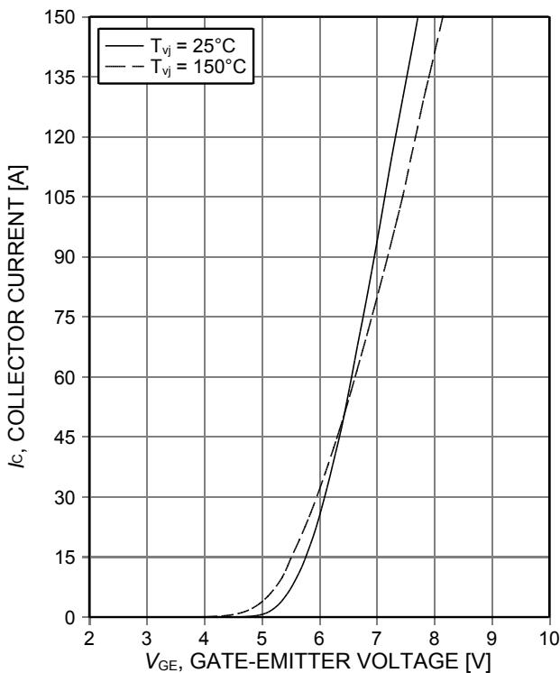
Figure 5. Typical transfer characteristic
