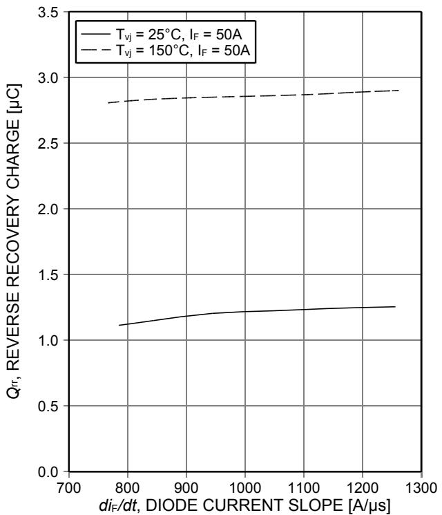
Figure 20. Typical reverse recovery charge as a function of diode current slope
