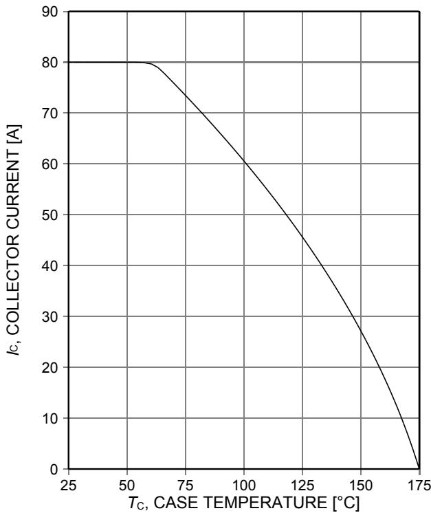
Figure 2. Collector current as a function of case temperature
