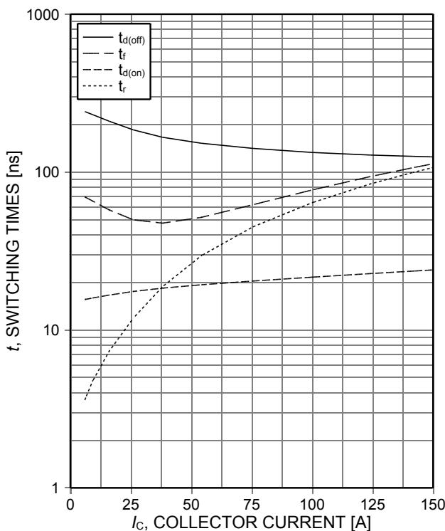
Figure 7. Typical switching times as a function of collector current
