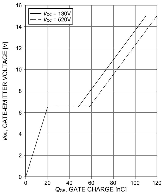
Figure 15. **Typical gate charge**
