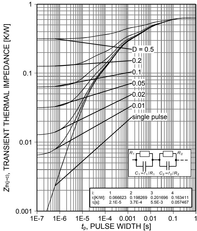
Figure 18. Diode transient thermal impedance as a function of pulse width
