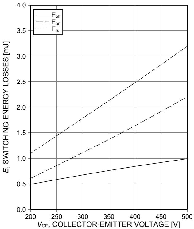
Figure 14. **Typical switching energy losses as a function of collector-emitter voltage**
