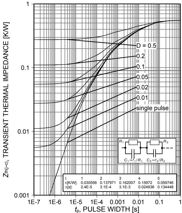
Figure 17. IGBT transient thermal impedance
