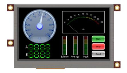
Embedded at the heart of the design is the **PICASO** processor, which is driven by a highly optimised virtual core engine called **EVE** (Extensible Virtual Engine). An extensive range of hardware and software peripherals have been integrated into the design, to give the user freedom to adapt the module to suit almost any application.
