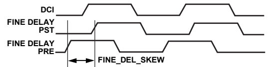
Figure 43. Pre- and Post-Delay Sampling Diagram
