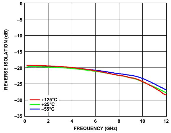
Figure 17. Reverse Isolation vs. Frequency, 200 MHz to 12 GHz, for Various Temperatures,  $V_{DD} = 5 V$ ,  $I_{DQ} = 55 \text{ mA}$
