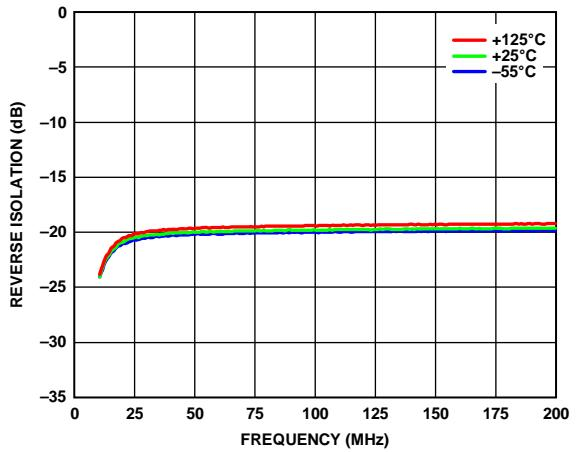
Figure 14. Reverse Isolation vs. Frequency, 10 MHz to 200 MHz, for Various Temperatures,  $V_{DD} = 5 V$ ,  $I_{DQ} = 55 \text{ mA}$
