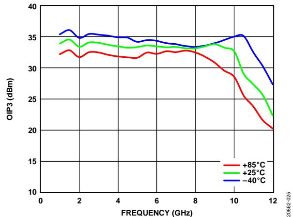
Figure 25. OIP3 vs. Frequency, 1 GHz to 12 GHz, for Various Temperatures,
