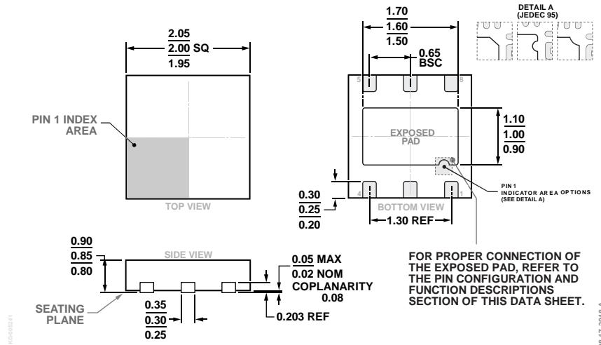
Figure 28. 6-Lead Lead Frame Chip Scale Package [LFCSP]
