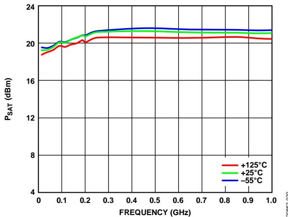
Figure 20.  $P_{SAT}$  vs. Frequency, 0.01 GHz to 1.0 GHz, for Various Temperatures,
