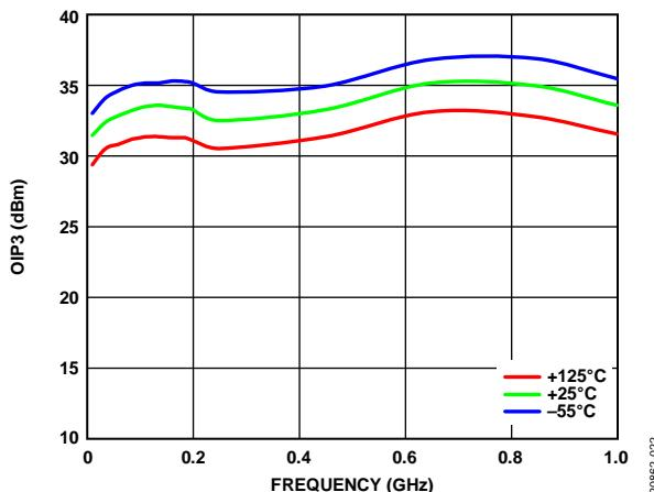
Figure 22. OIP3 vs. Frequency, 0.01 GHz to 1.0 GHz, for Various Temperatures,
