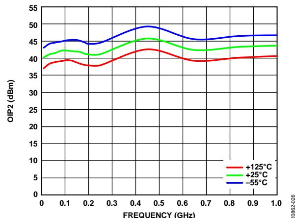
Figure 26. OIP2 vs. Frequency, 0.01 GHz to 1.0 GHz, for Various Temperatures,
