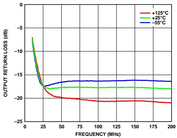
Figure 10. Output Return Loss vs. Frequency, 10 MHz to 200 MHz,
