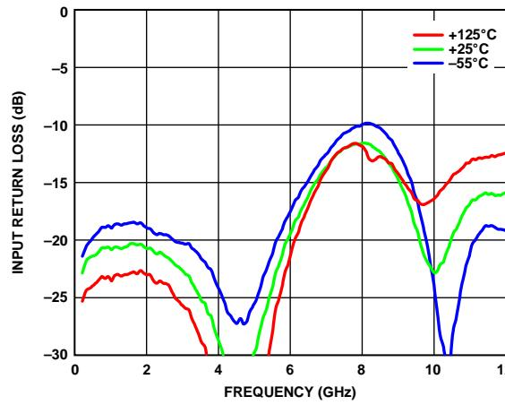
Figure 12. Input Return Loss vs. Frequency, 200 MHz to 12 GHz,
