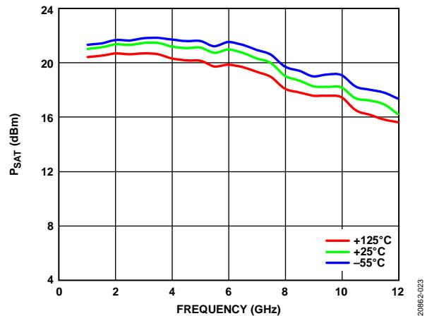
Figure 23.  $P_{SAT}$  vs. Frequency, 1 GHz to 12 GHz, for Various Temperatures,
