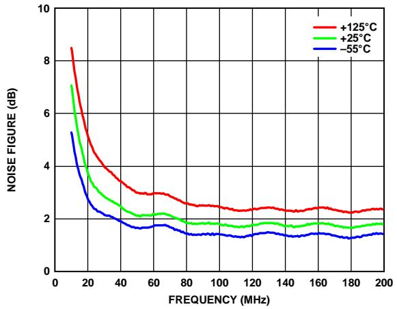
Figure 15. Noise Figure vs. Frequency, 10 MHz to 200 MHz, for Various Temperatures,  $V_{DD} = 5 V$ ,  $I_{DQ} = 55 \text{ mA}$
