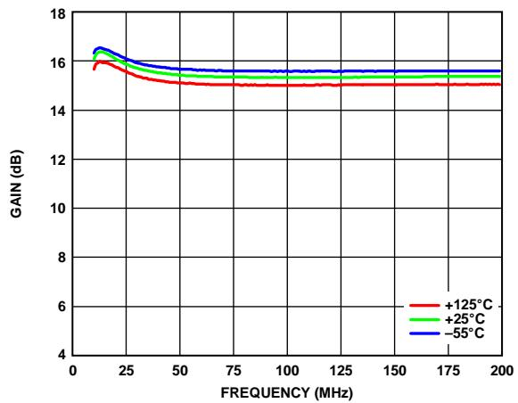
Figure 8. Gain vs. Frequency, 10 MHz to 200 MHz, for Various Temperatures,
