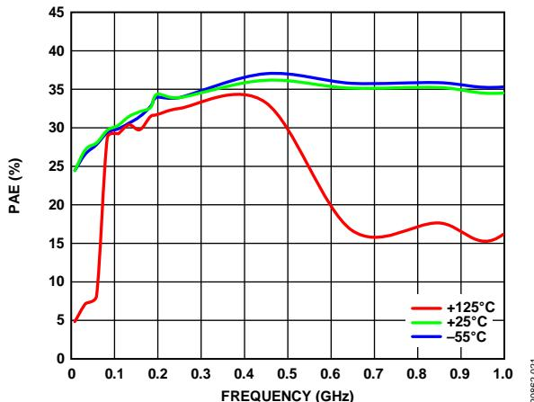
Figure 21. PAE vs. Frequency, 0.01 GHz to 1.0 GHz, for Various Temperatures,
