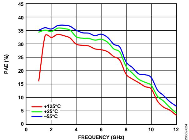
Figure 24. PAE vs. Frequency, 1 GHz to 12 GHz, for Various Temperatures,
