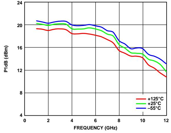
Figure 19. P1dB vs. Frequency, 1 GHz to 12 GHz, for Various Temperatures,  $V_{DD} = 5 V$ ,  $I_{DQ} = 55 \text{ mA}$
