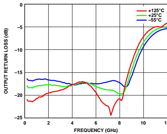
Figure 13. Output Return Loss vs. Frequency, 200 MHz to 12 GHz,
