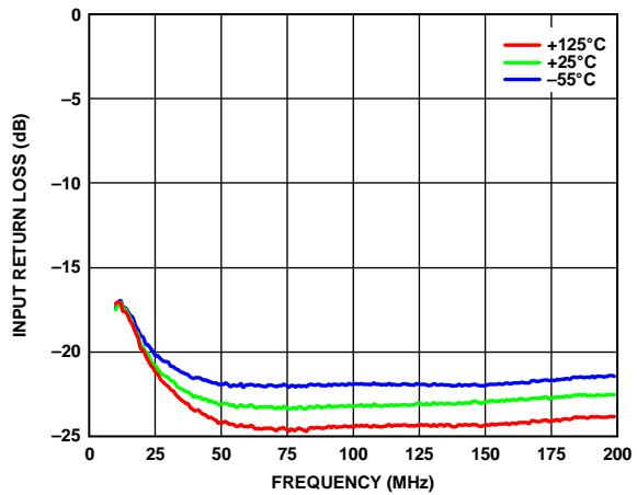
Figure 9. Input Return Loss vs. Frequency, 10 MHz to 200 MHz,
