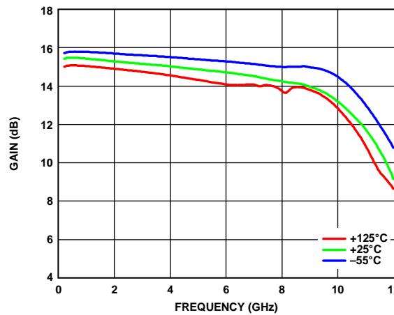
Figure 11. Gain vs. Frequency, 200 MHz to 12 GHz, for Various Temperatures,
