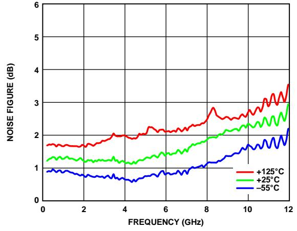
Figure 18. Noise Figure vs. Frequency, 200 MHz to 12 GHz, for Various Temperatures,  $V_{DD} = 5 V$ ,  $I_{DQ} = 55 \text{ mA}$
