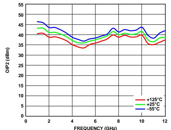
Figure 27. OIP2 vs. Frequency, 1 GHz to 12 GHz, for Various Temperatures,
