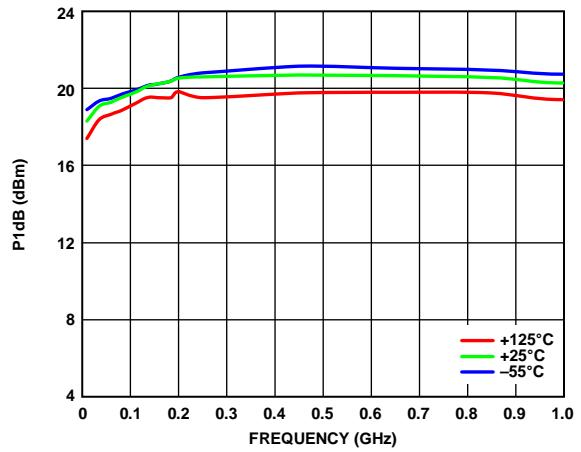
Figure 16. P1dB vs. Frequency, 0.01 GHz to 1.0 GHz, for Various Temperatures,  $V_{DD} = 5 V$ ,  $I_{DQ} = 55 \text{ mA}$
