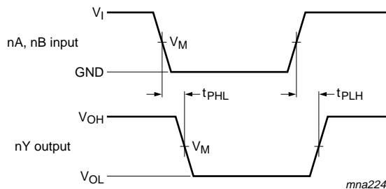
Measurement points are given in [Table 8](#).V<sub>OL</sub> and V<sub>OH</sub> are typical voltage output levels that occur with the output load.**Fig 6. Input to output propagation delays****Table 8. Measurement points**
