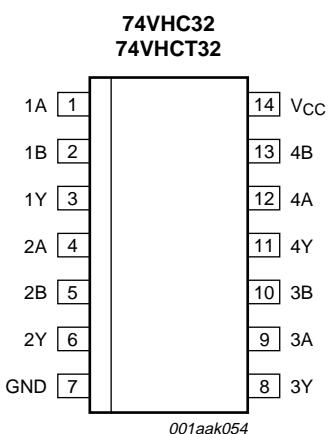
Fig 4. Pin configuration SO14 and TSSOP14
