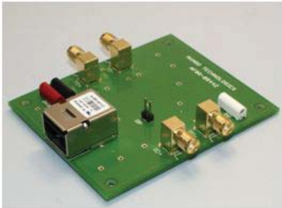
Figure 1. Evaluation board for the AFBR-5972Z transceiver module
